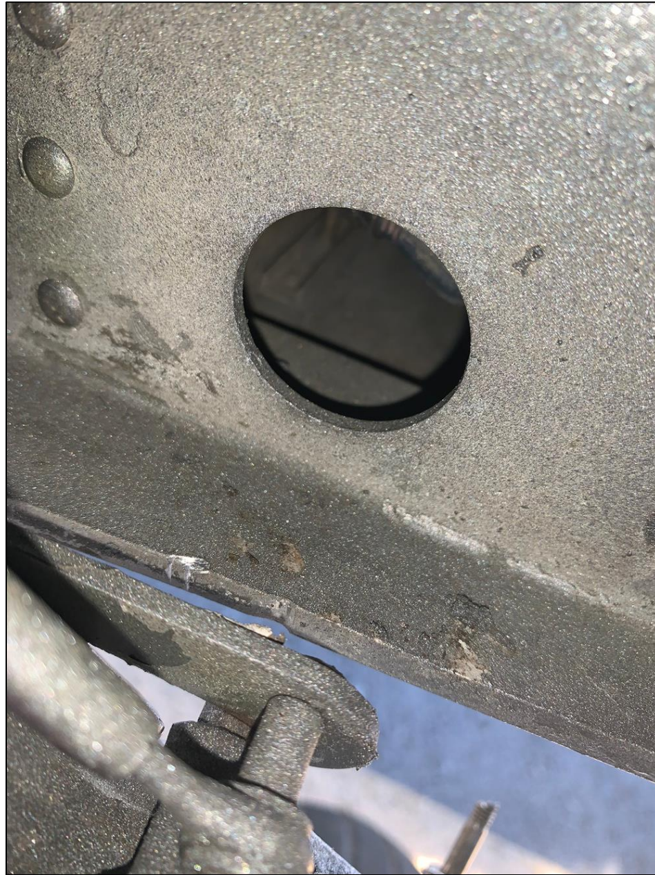
Photo 4 – Mechanical damage inside of right main landing gear wheel well. (Courtesy of the insurance adjuster)
