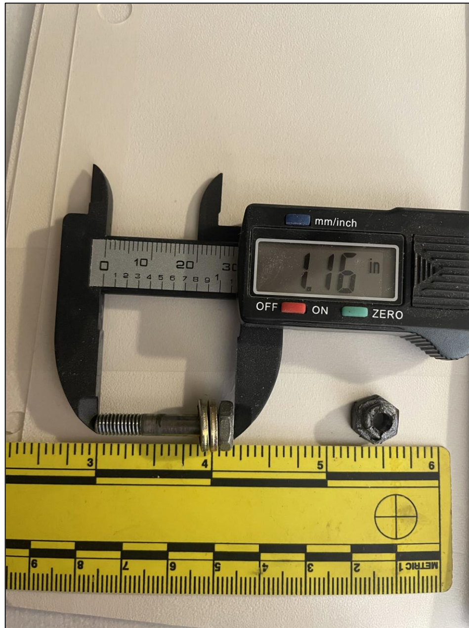
Photo 3 - Right main landing gear door rod-end bolt. (Photo courtesy of the NTSB-IIC)
