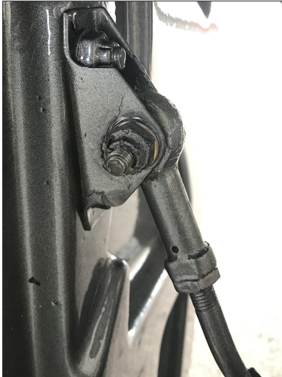
Photo 1 – Right main landing gear door rod-end bolt. (Photo courtesy of a hired mechanic)
