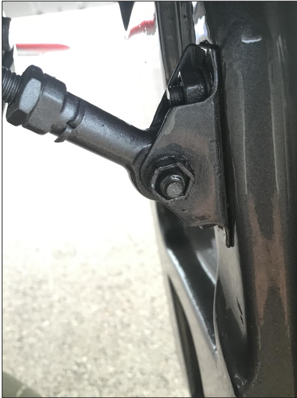
Photo 2 - Left main landing gear door rod-end bolt. (Photo courtesy of a hired mechanic)
