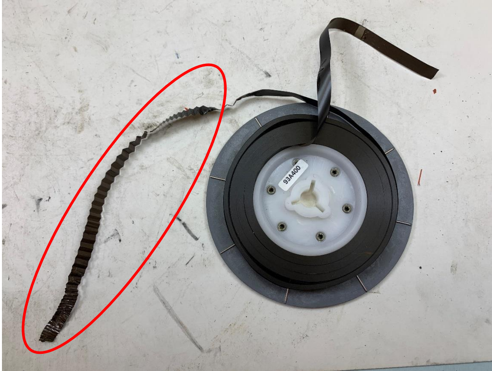
Figure 4. The magnetic tape, liberated from the recording mechanism, showing operational damage.
