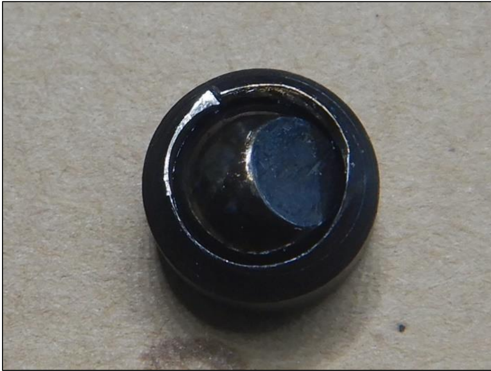
Figure 4-Rocker valve swivel pad and housing (valve side view).
