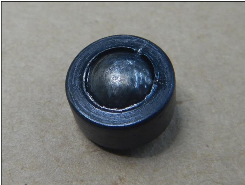
Figure 5-Rocker valve swivel pad and housing (separated section view)
