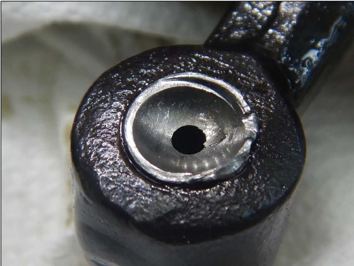
Figure 6-Rocker and swivel adjustment screw section.
