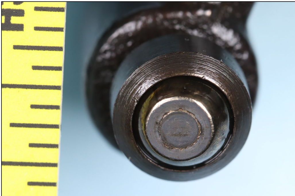
Figure 9. Number 3 exhaust valve adjuster showing spalling damage on the swivel pad face.
