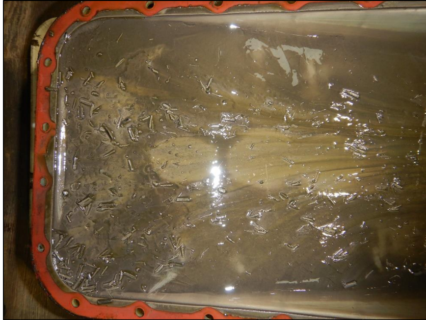
Figure 8-Oil sump and contents.
