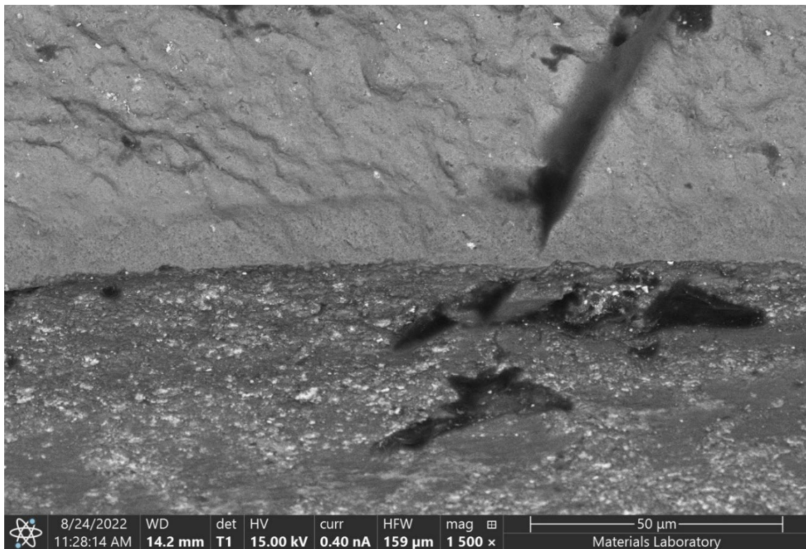
Figure 19. BE micrograph highlighting a closer view of the initiation site in Figure 18.
