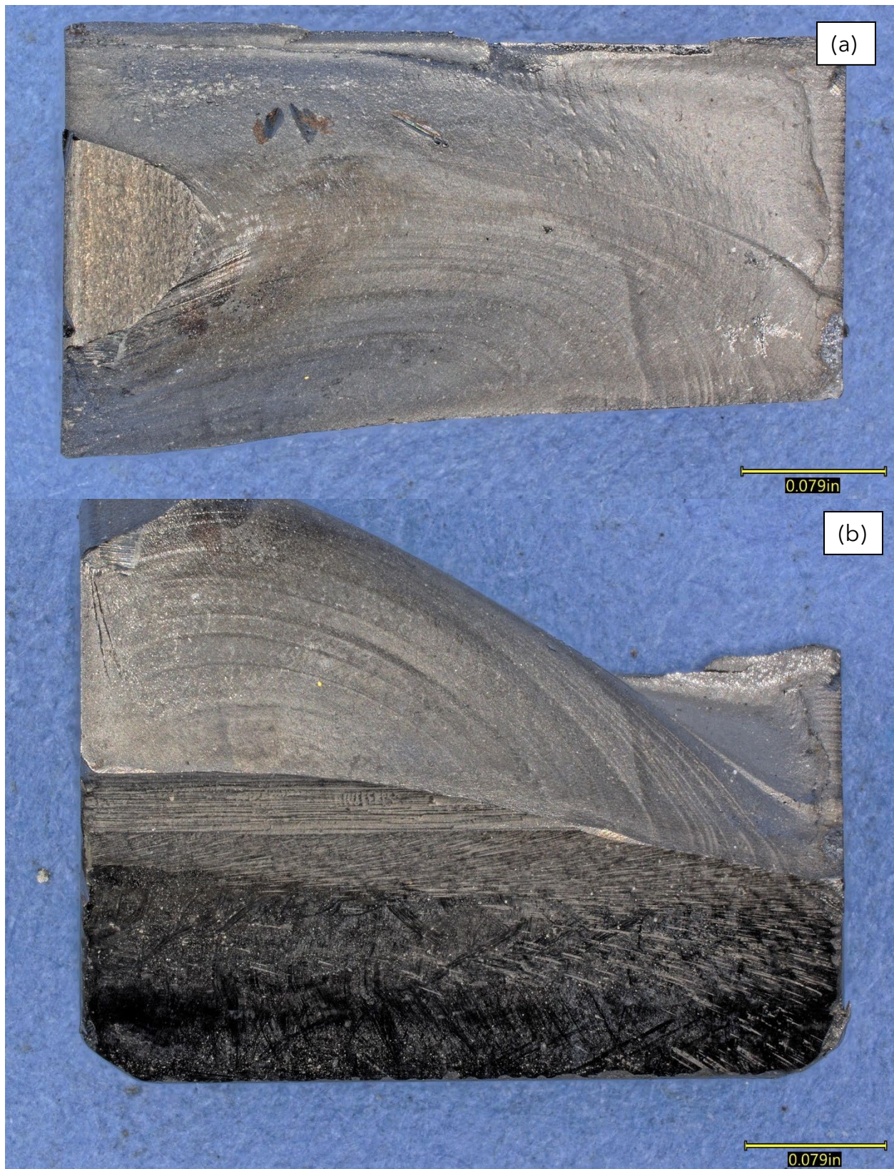
Figure 15. Views of the fractured gear tooth #4, viewed from (a) the fracture surface and (b) the side.
