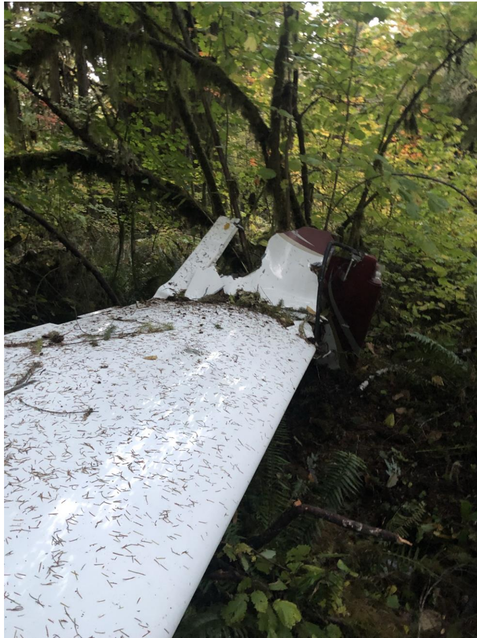
Photo 4 – Accident site, left wing damage. (Courtesy of airplane owner)
