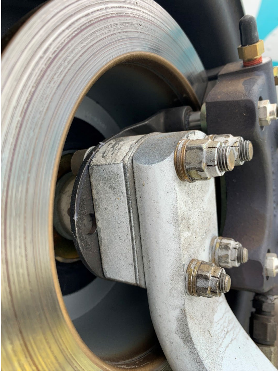
Figure 6. Left main landing gear with shim. Photo FAA.
