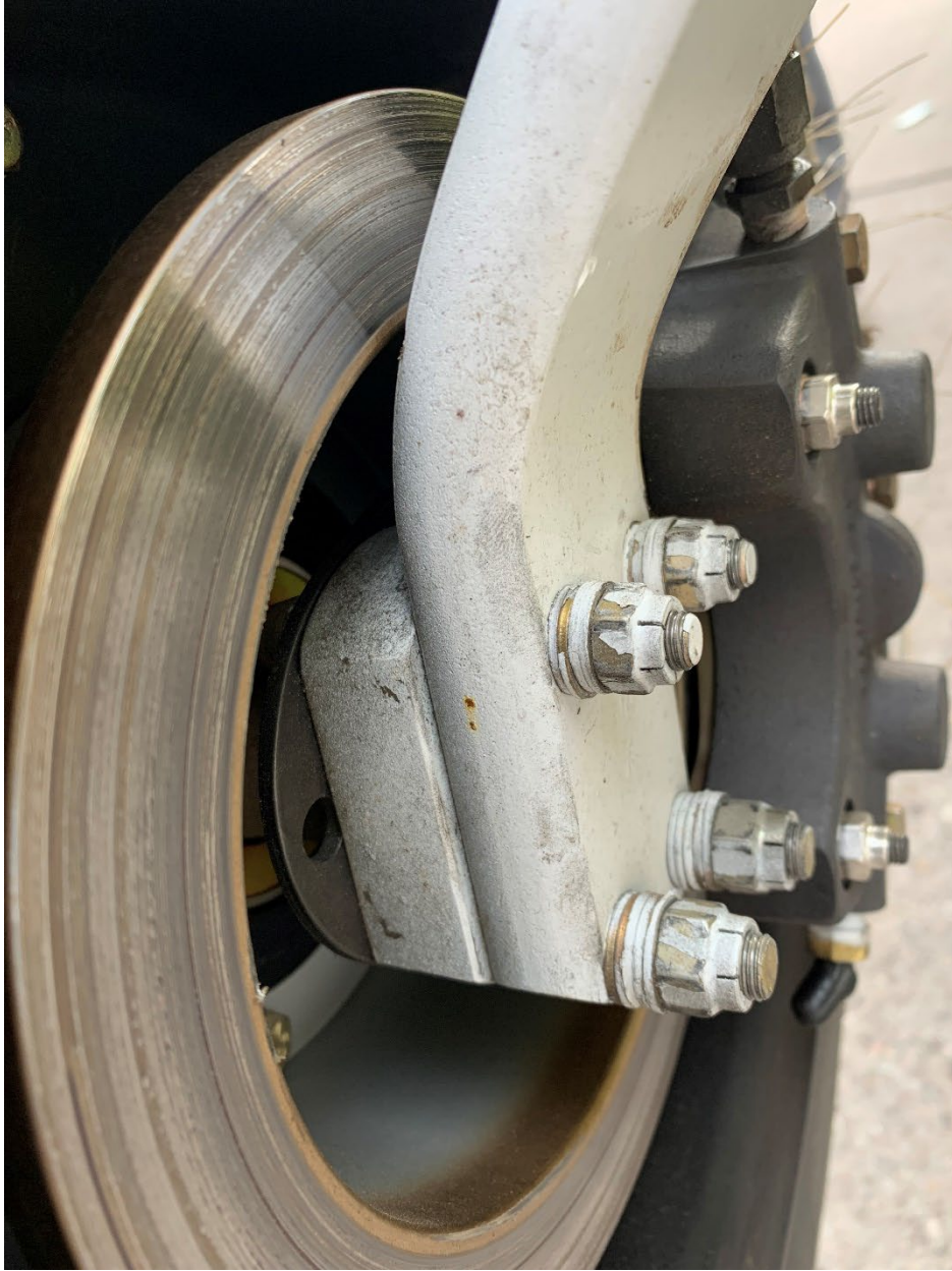
Figure 7. Right main landing gear without shim. Photo FAA.
