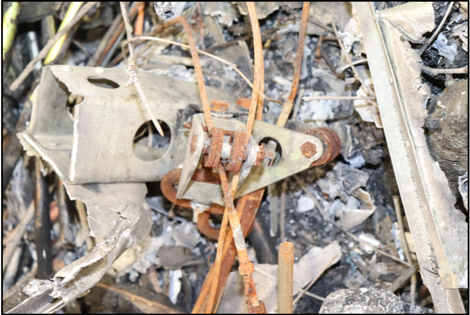
Figure 10: No. 9 Pulley with Hook Attachment
