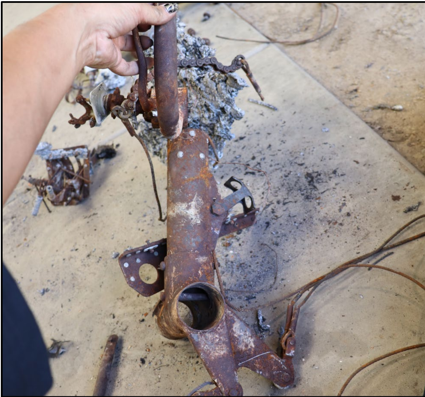
Figure 4: Aileron Chain and Elevator Cable Connections at the Control Column
