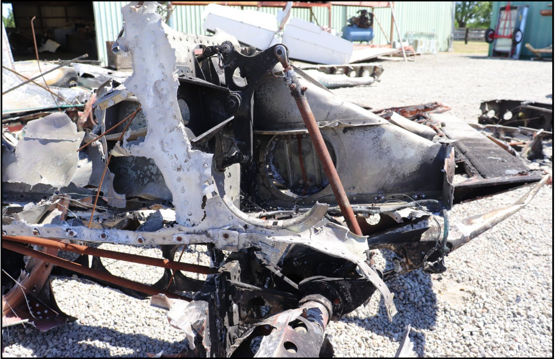
Figure 13: Control Tubes to Elevator
