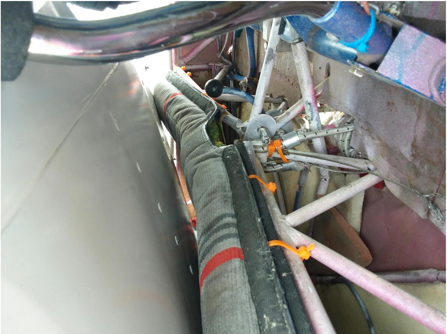
Photo 2 – View of the airplane’s structural damage, lower cabin area. (Courtesy of the FAA)
