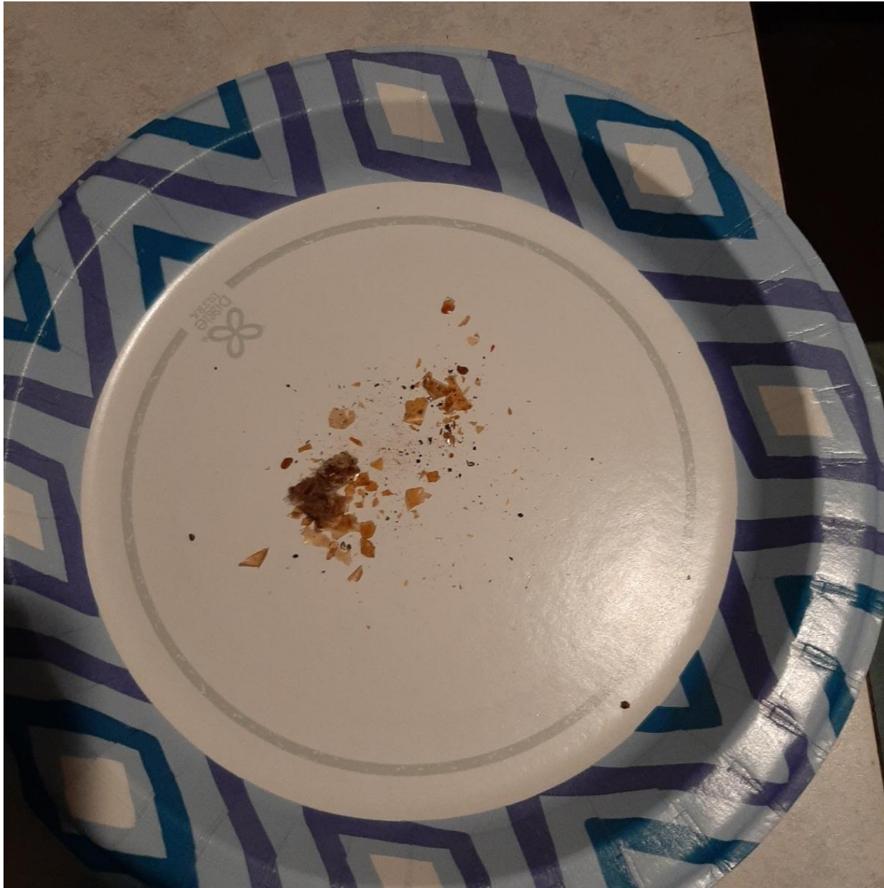
Photo 4 – Debris found in the fuel selector valve. (Courtesy of the FAA)
