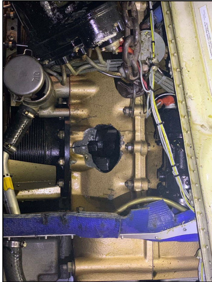
Figure 1: Hole in engine as viewed from the top.
