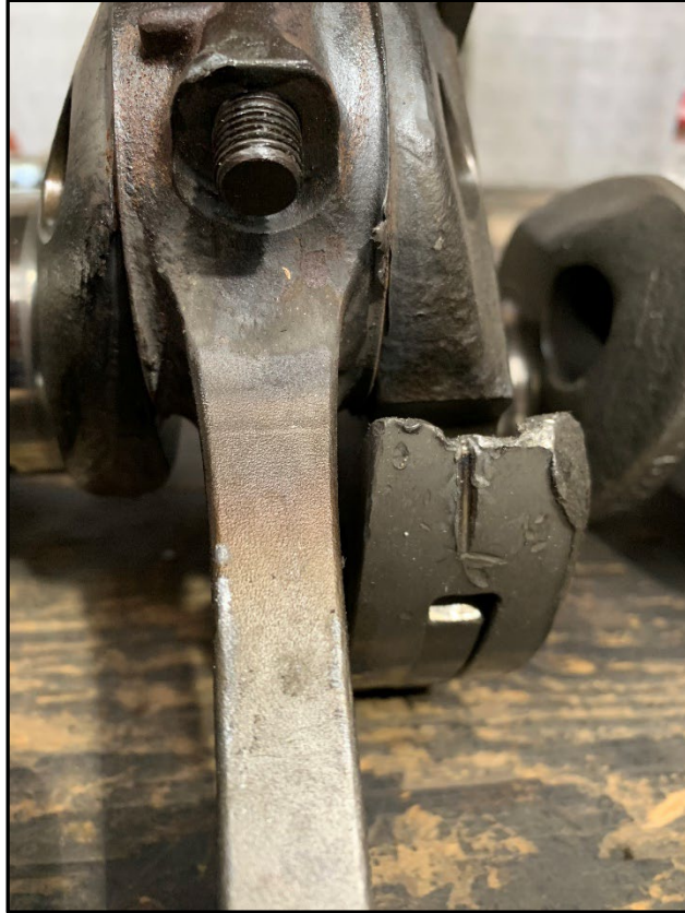
Figure 3: No. 4 Connecting Rod Bolt nut missing.
