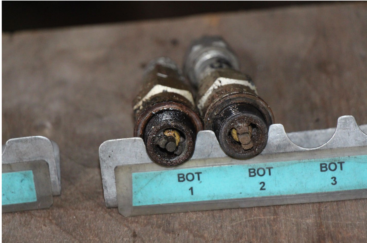
Photograph 5: Bottom spark plugs
