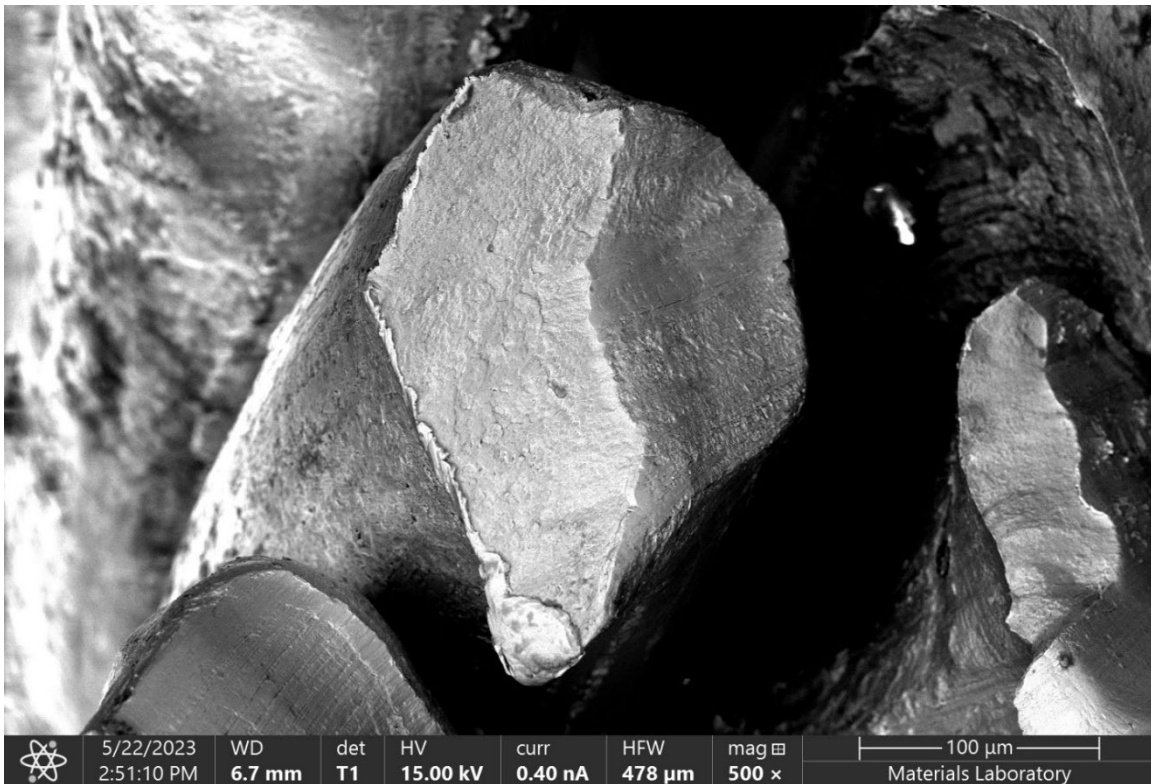
Figure 21. BE micrograph of a deformed wire from Strand 4 in Figure 20 .
