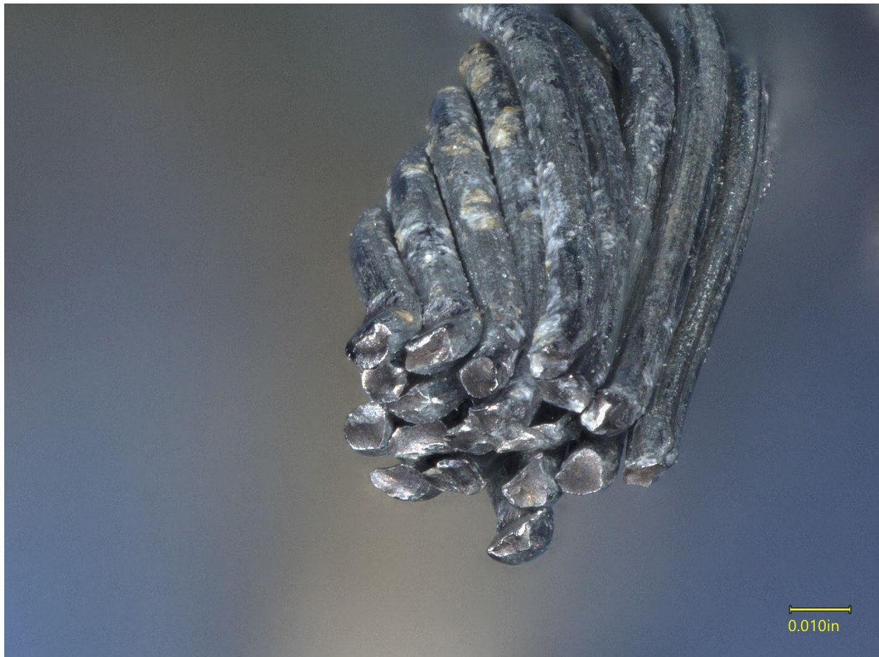
Figure 8. View of the fractured wire ends of strand 3 from the left cable.
