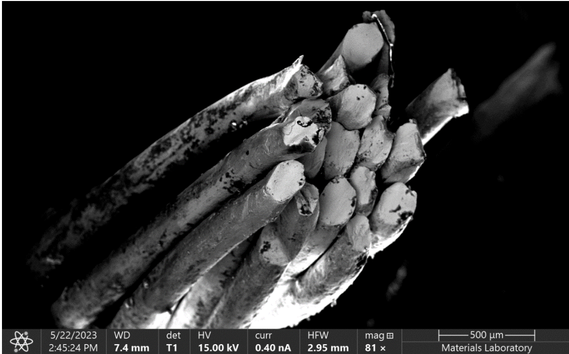
Figure 12. Backscattered electron (BE) micrograph of strand 3 fractured wire surfaces from the left cable.
