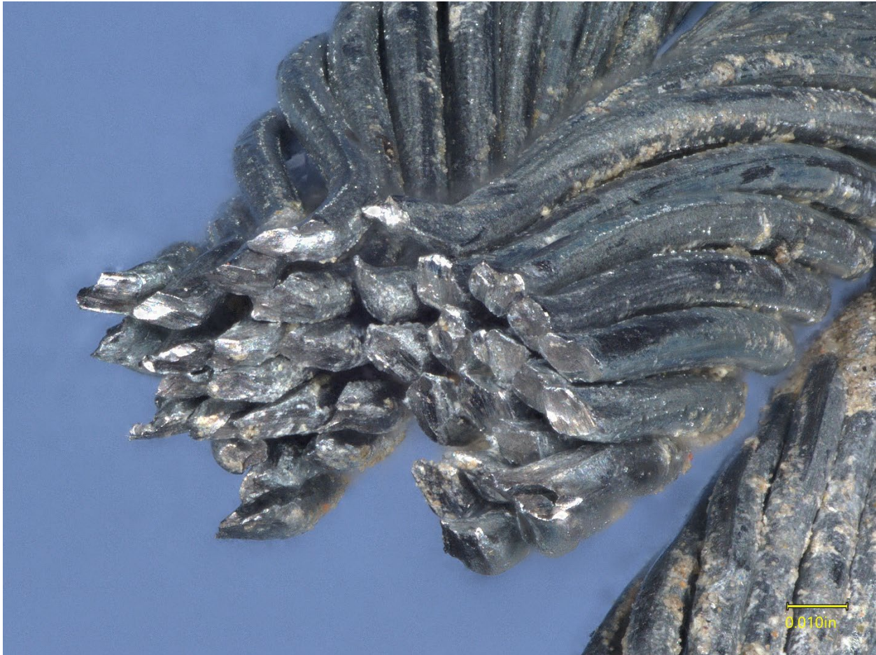
Figure 9. Slanted fracture surfaces of the wires from strands 4 and 5 from the left aileron control cable.
