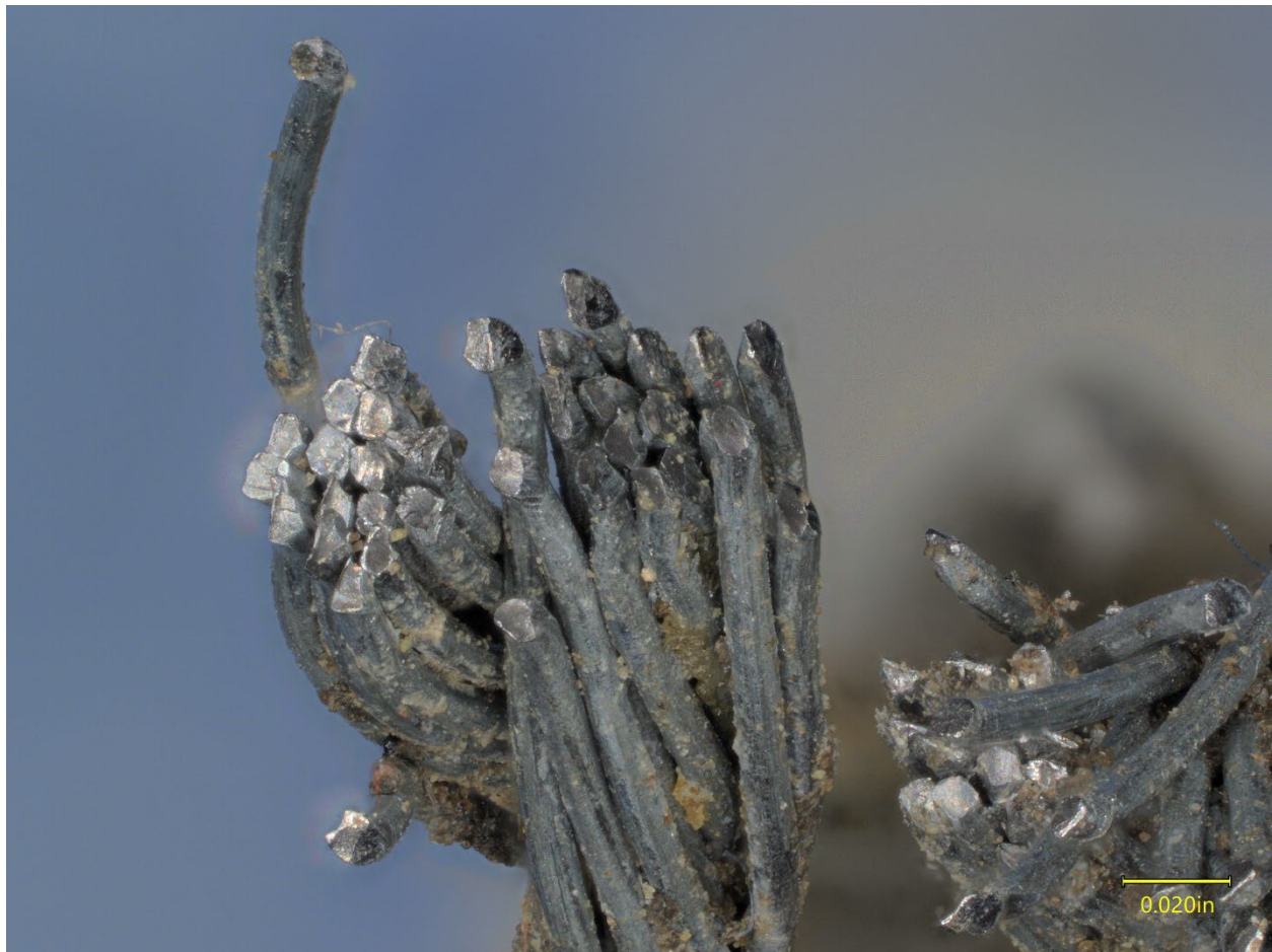
Figure 26. The fractured ends of strands 5 and 6 from the right aileron cable.
