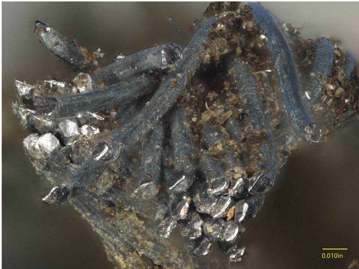
Figure 25. The fractured ends of strands 2 and 3 from the right aileron cable.
