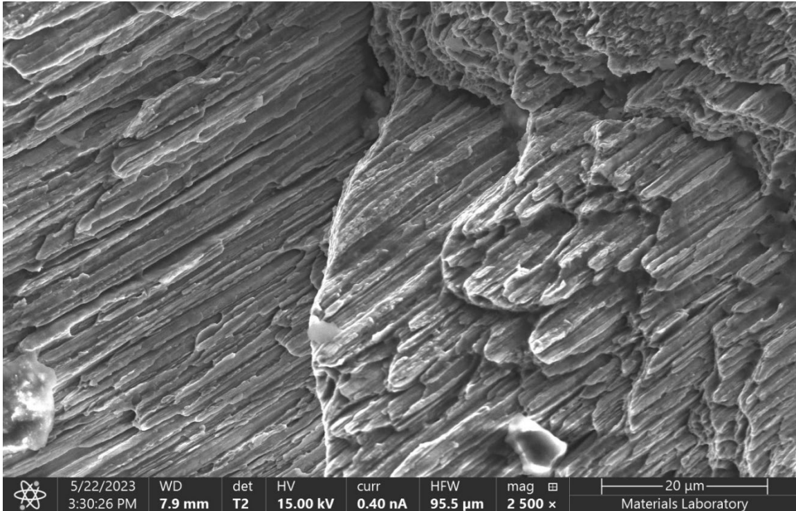
Figure 31. BE micrograph of the upper right wire fracture surface in Figure 30 , showing ductile tearing and dimpled rupture along the elongated grain direction.
