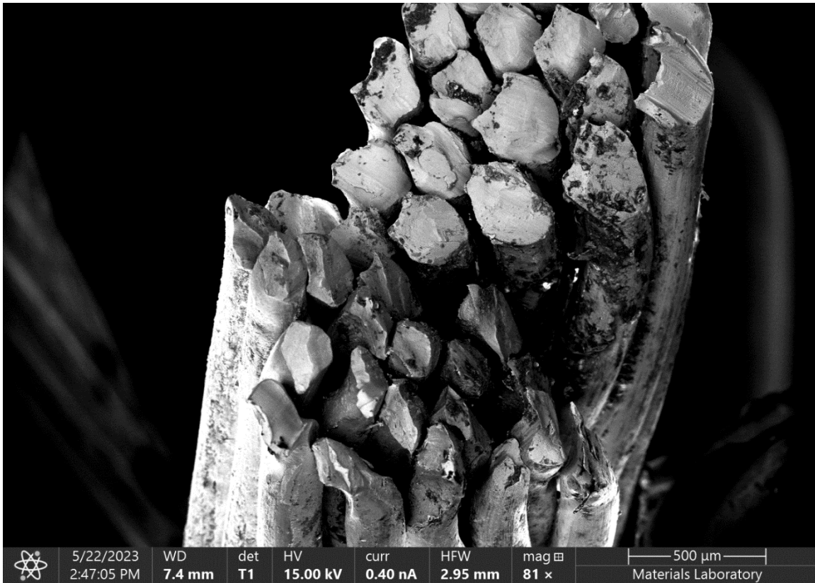
Figure 20. BE micrograph of the fourth and fifth wire strands from the left cable.
