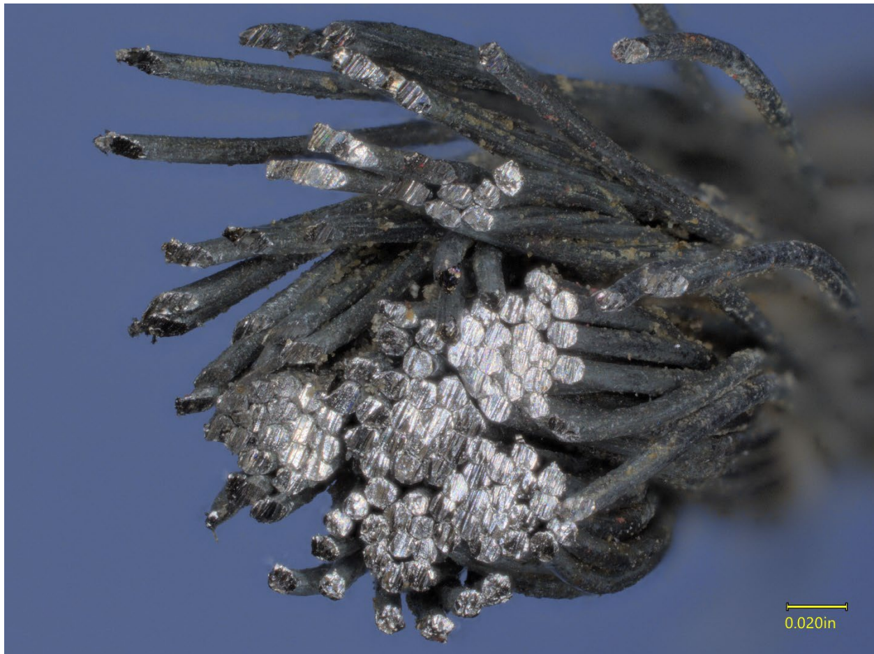
Figure 11. Comparative view of the opposite cut and sectioned wires from the left aileron cable, shown for comparison to the fractured end.
