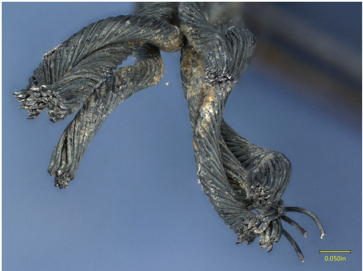
Figure 4. The fractured wire ends of the strands of the left aileron cable.
