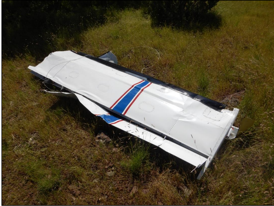
Figure 8-Right outboard wing section.
