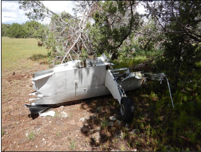
Figure 4-Left inboard wing section.
