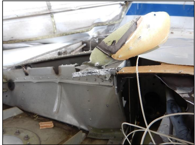
Figure 7-Right wing main spar separation.
