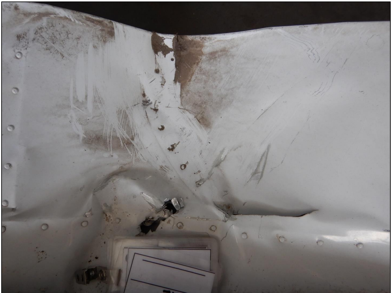
Figure 4-The left aileron rivet imprint.
