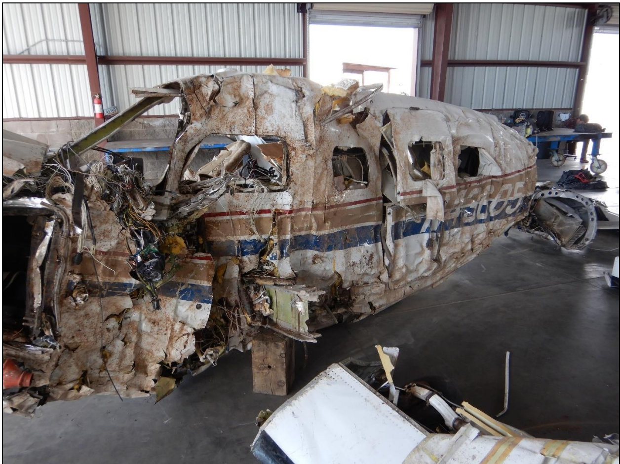
Figure 1-The left side of the fuselage and left wing spar inboard section.
