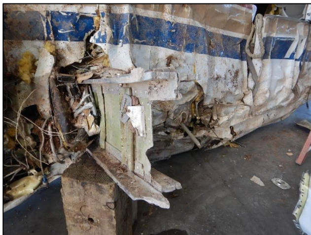
Figure 2-The left main wing spar separation.
