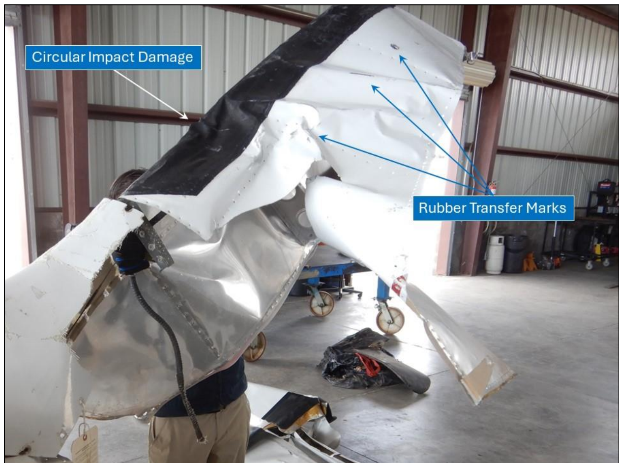
Figure 6-Vertical stabilizer skin held in place relative to its normal position on the empennage.
