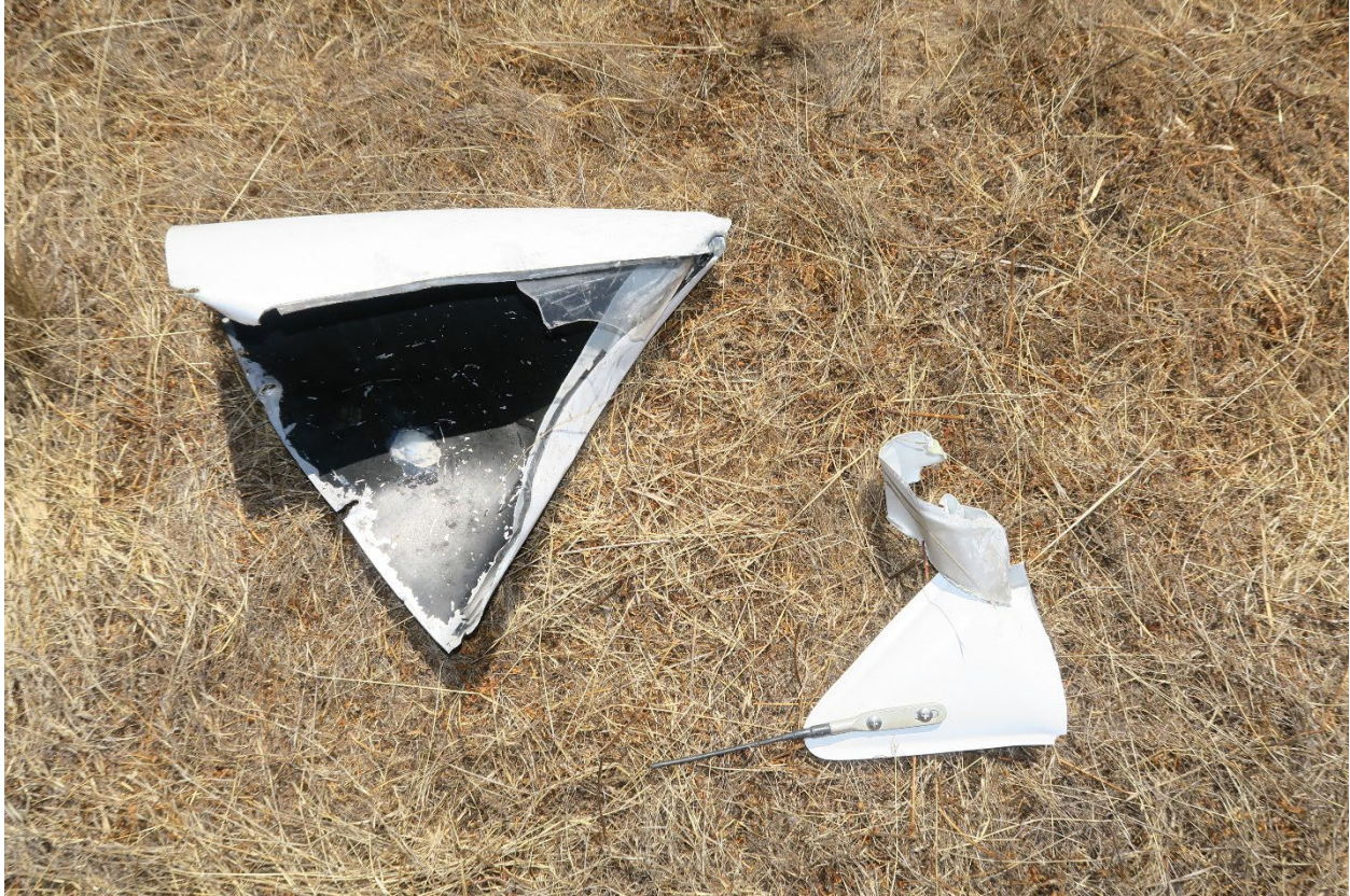
Figure 26. Two sections of the Cessna 340's left-wing tip tank. Photo Textron.
