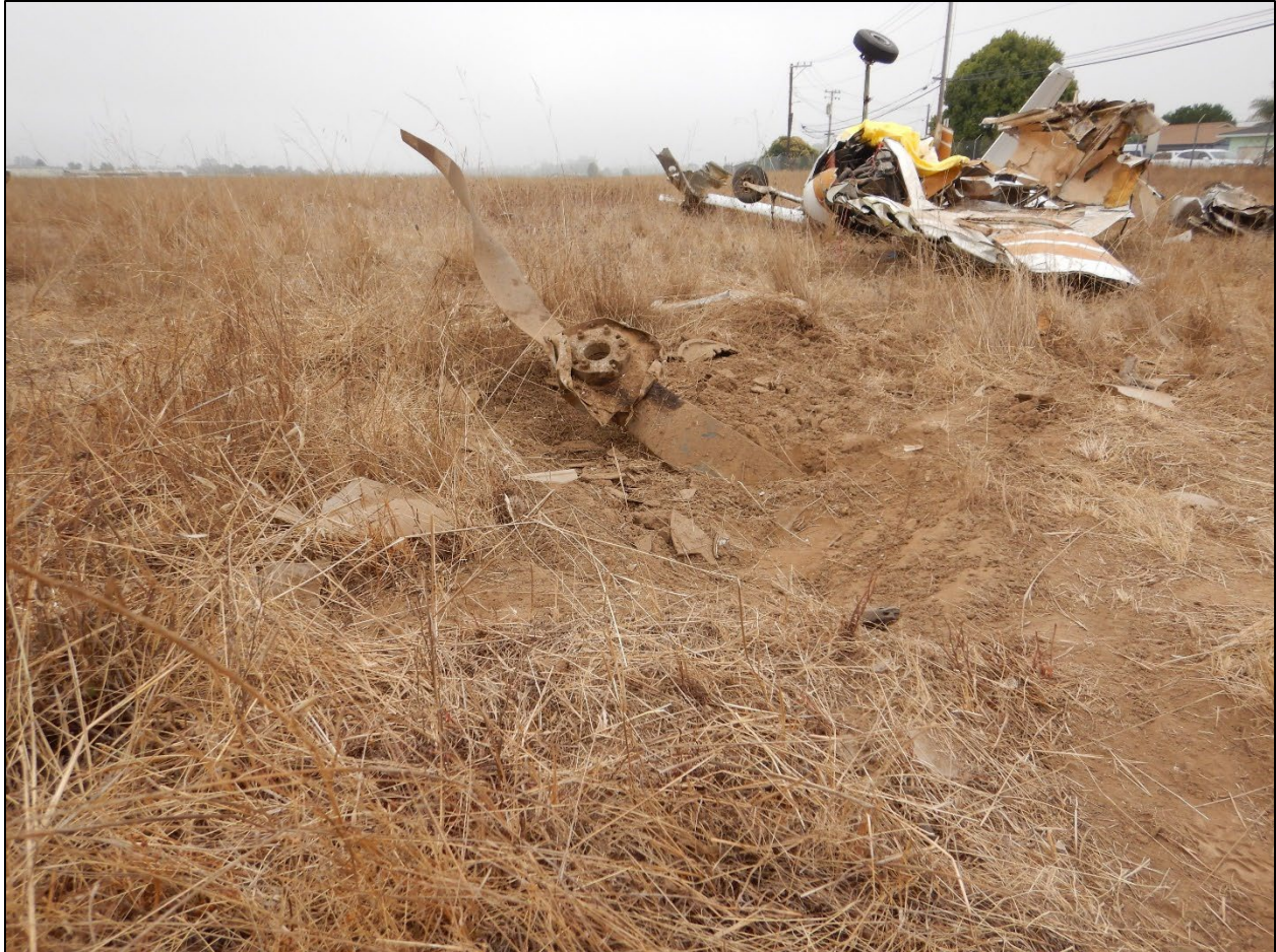
Figure 18-Accident site, view to the southwest, impact crater and Cessna 152 main wreckage.
