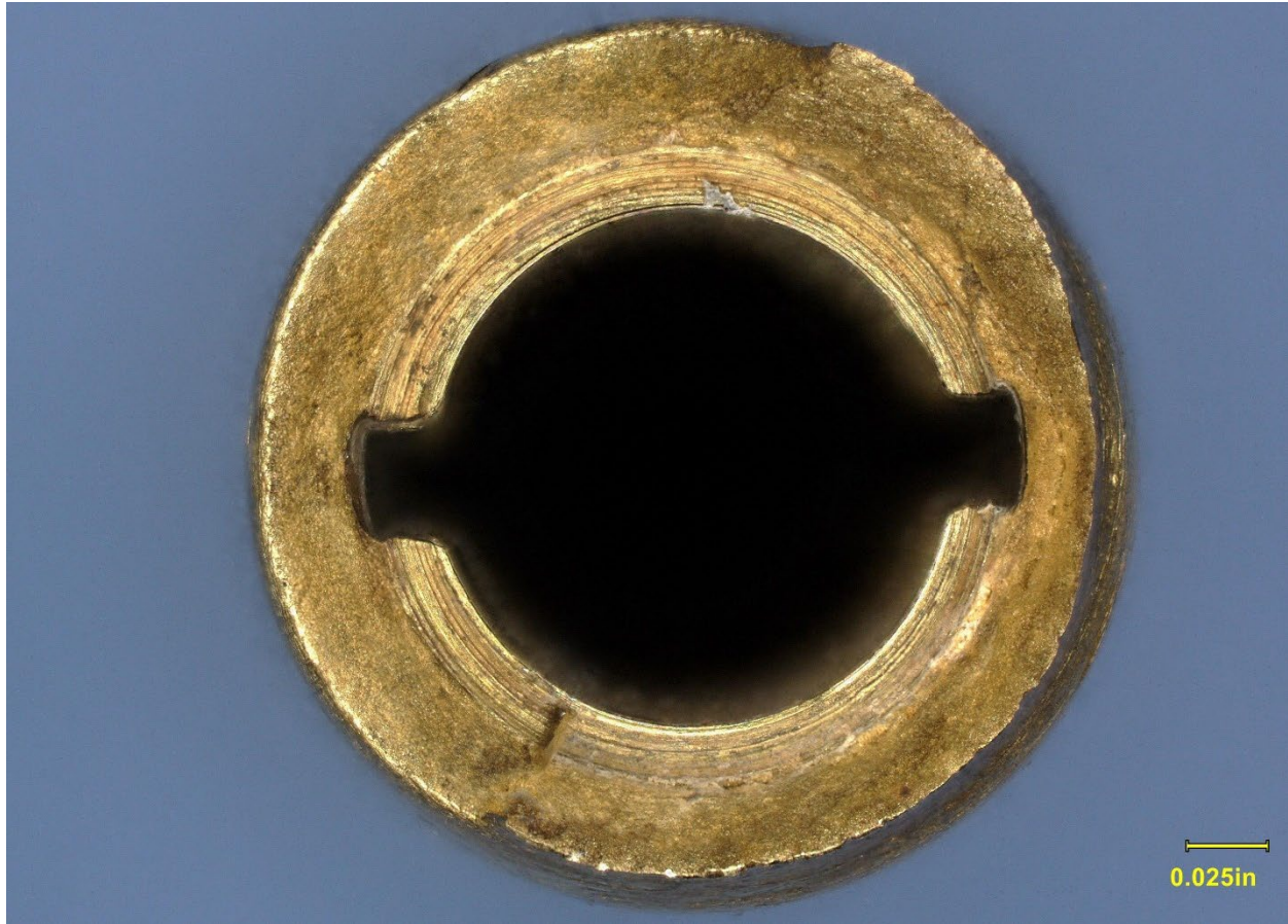
Figure 5. View of the fracture surface of the smaller turnbuckle remnant on the right in Figure 4 .
