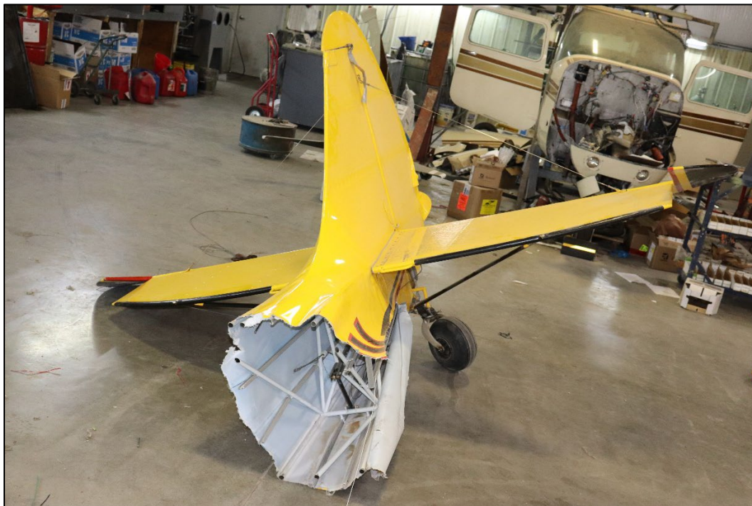
Figure 4: View of empennage during examination
