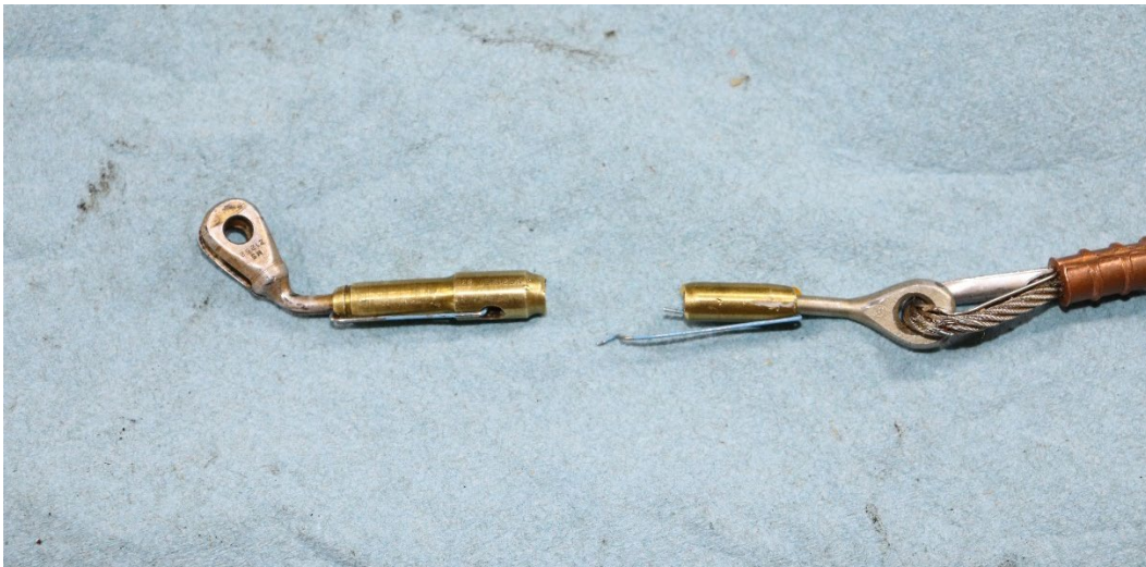
Figure 14: View of damaged turnbuckle barrel
