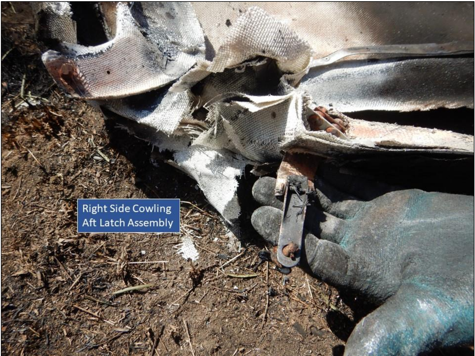
Photograph 6 - Accident site, upper cowling right aft latch.
