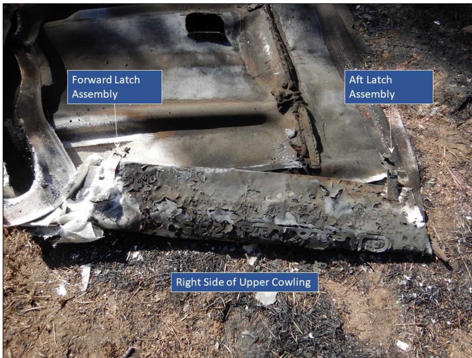
Photograph 5 - Accident site, upper cowling.
