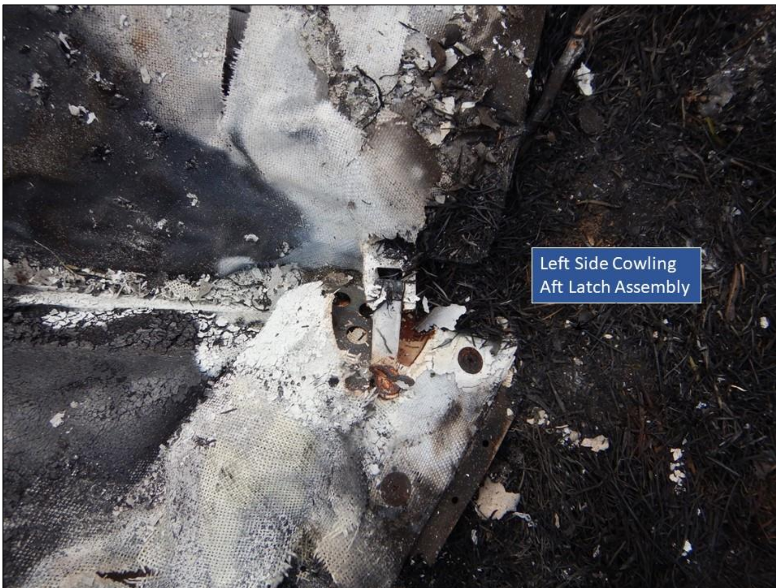
Photograph 7 - Accident site, upper cowling left aft latch.
