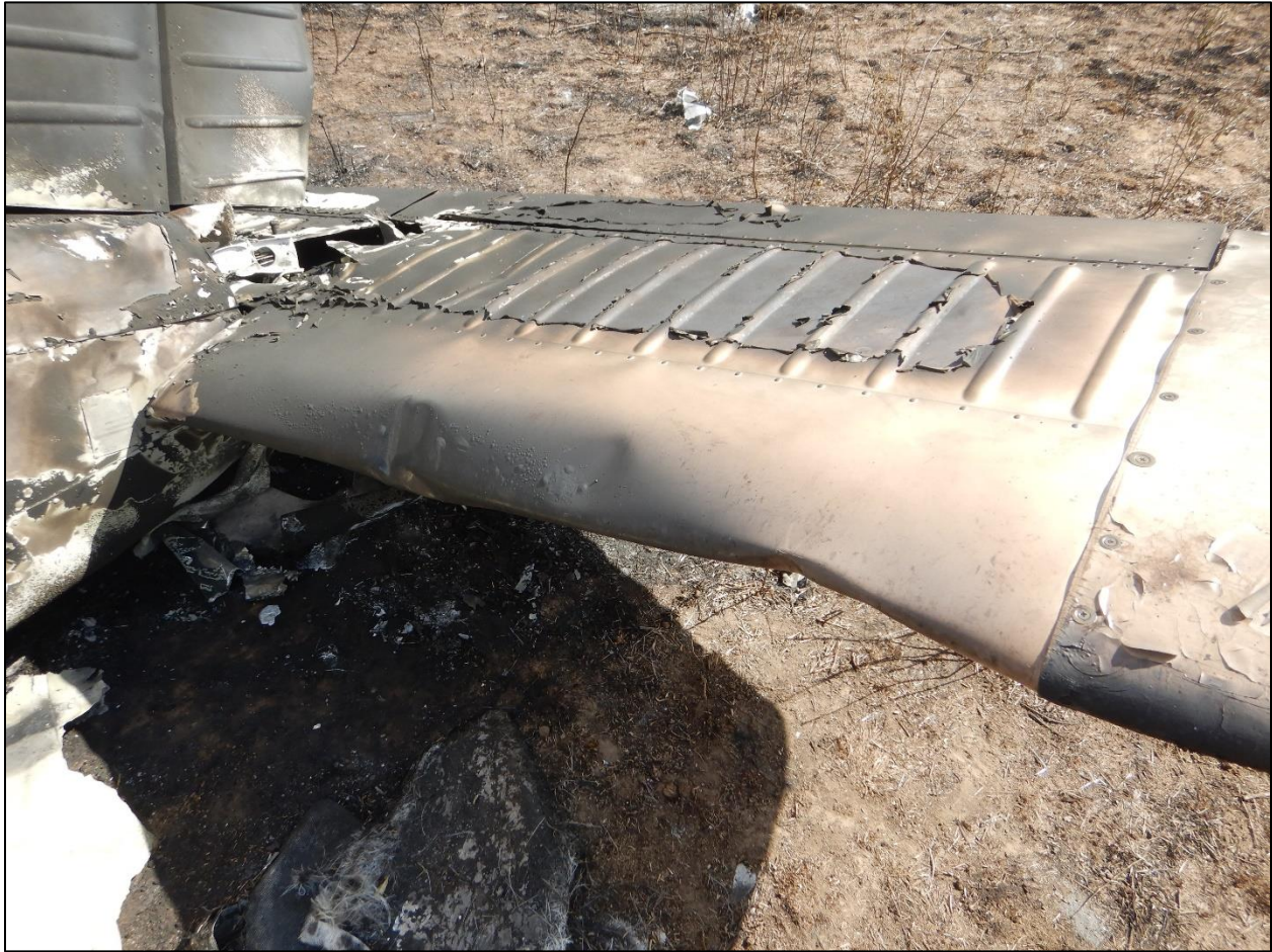
Figure 4-View of the left horizontal stabilizer.
