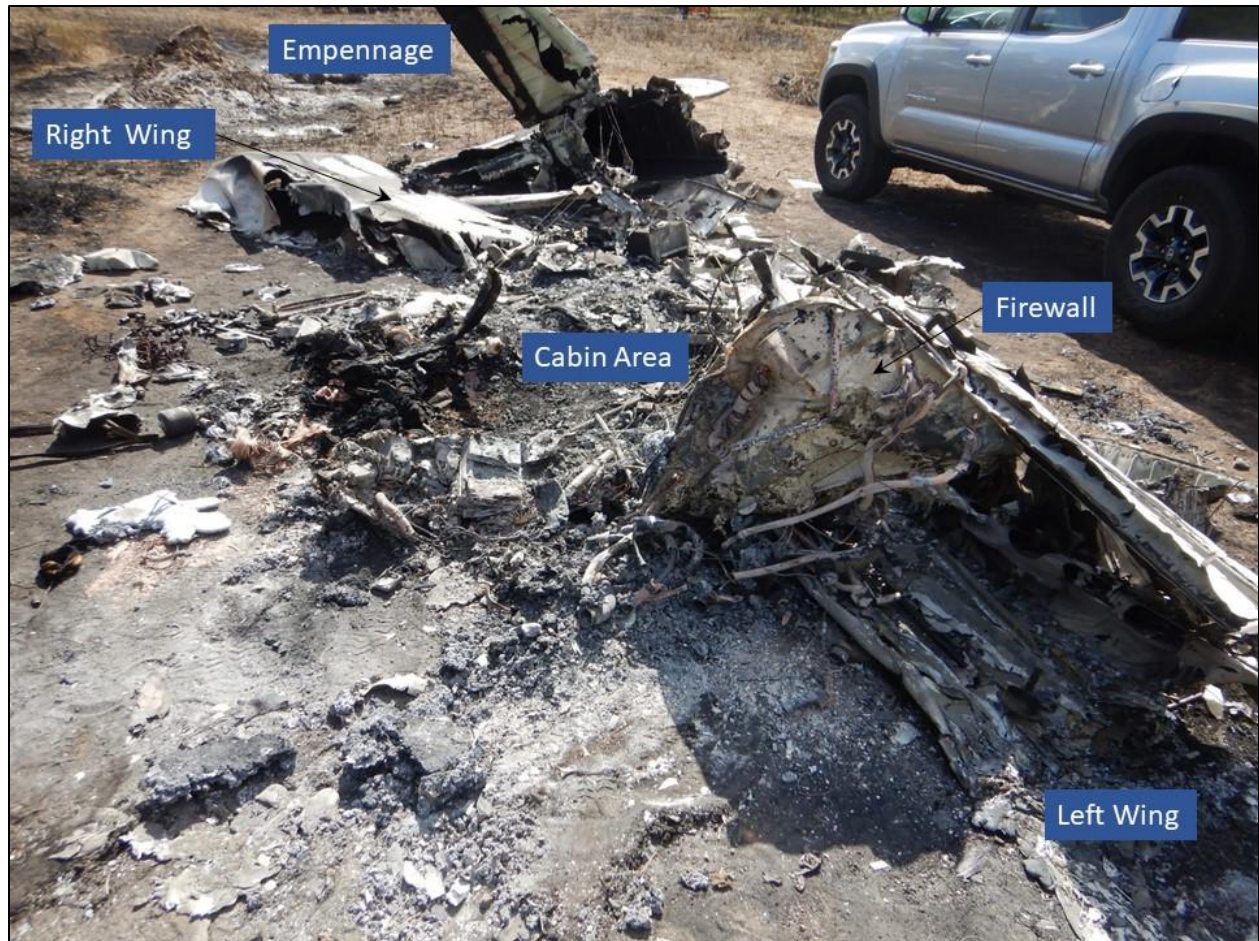
Figure 5-Main wreckage, cabin and wings.
