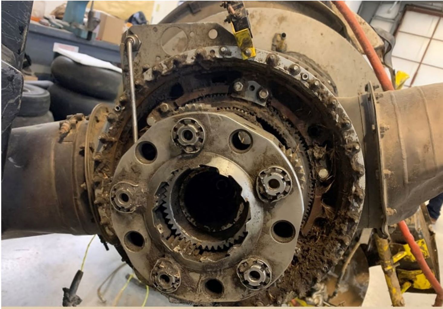
Photograph 4 - View of reduction gearbox "A" flange fracture
