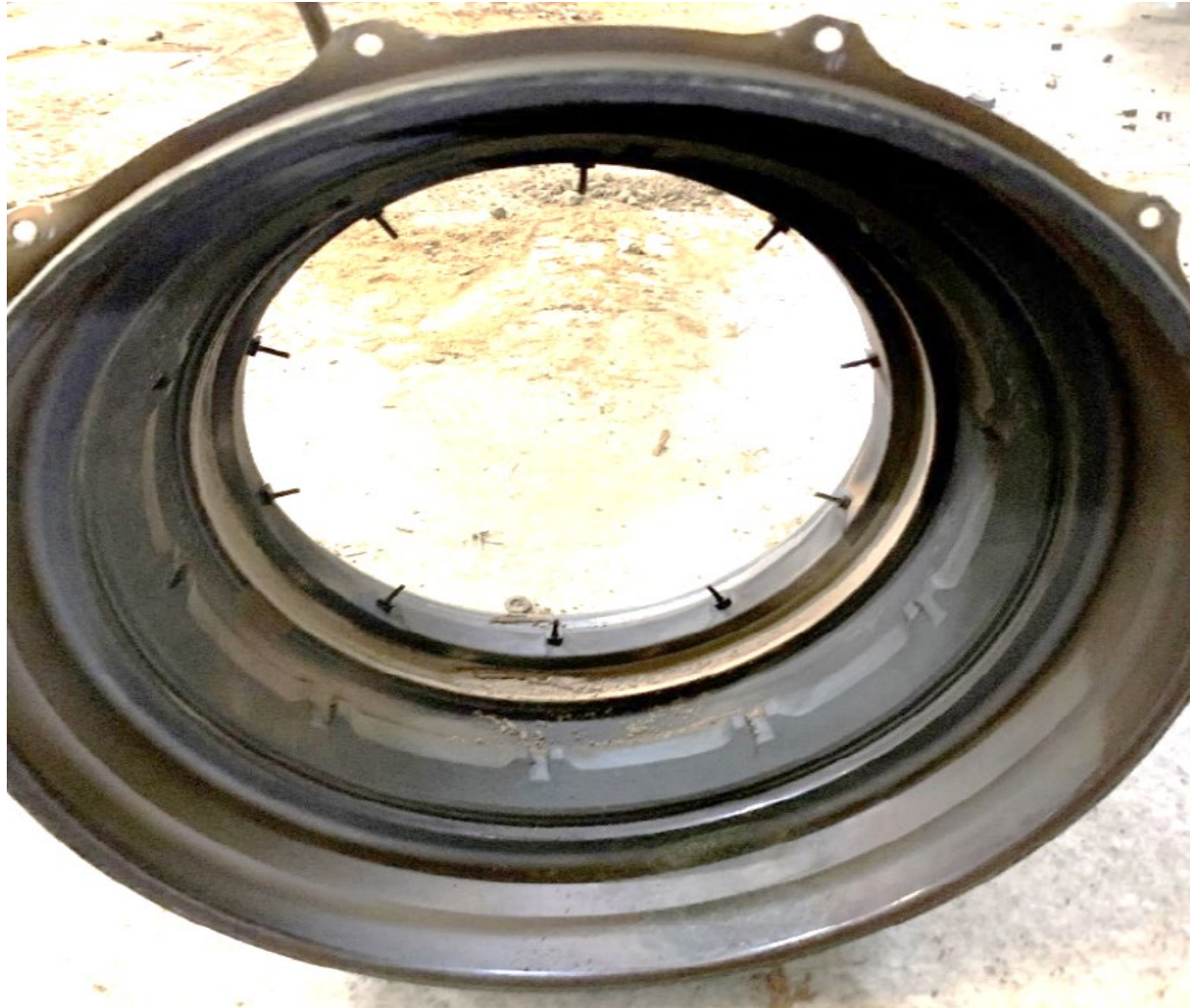
Photograph 3 - View of Power Turbine stator housing with environmental debris
