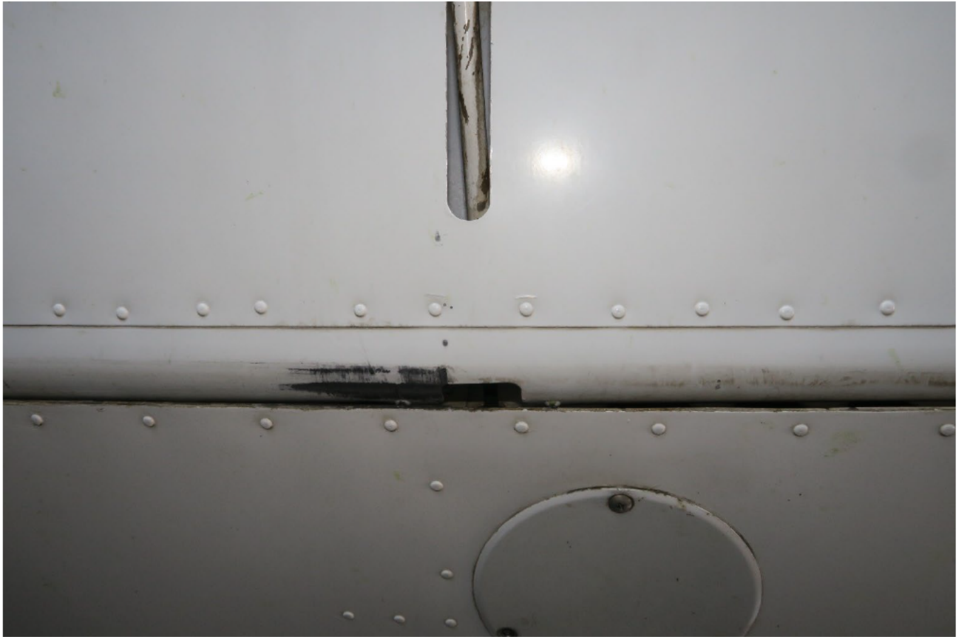
Wreckage Exam ASI-22-BK-029 (chaffing area of right horizontal stabilizer and elevator)
