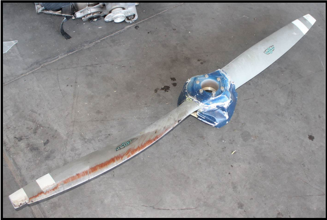
Figure 3: N934JH Propeller removed for engine examination
