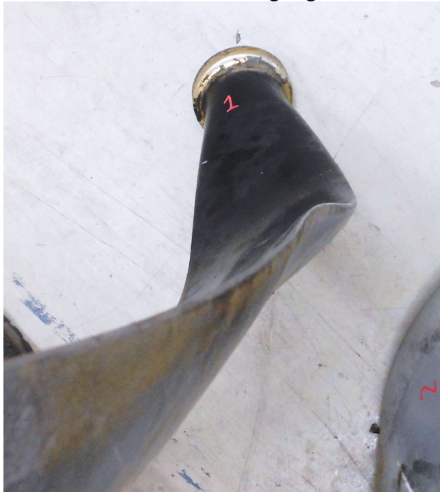
Photo #17 - Blade #1 leading edge wave bend
