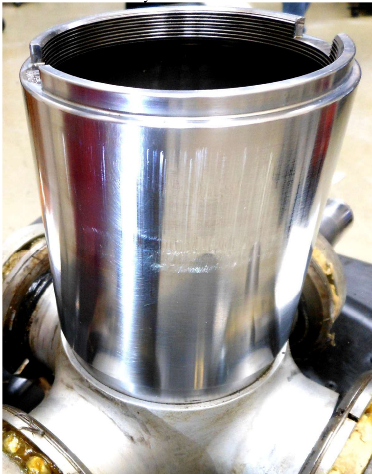
Photo #8 - Cylinder surface scuff marks
