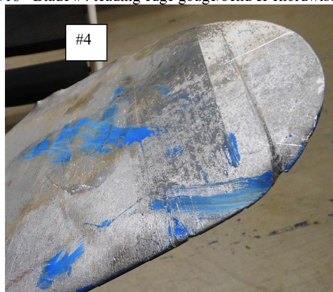
Photo #16 - Blade #4 leading edge gouge/bend & chordwise scoring
