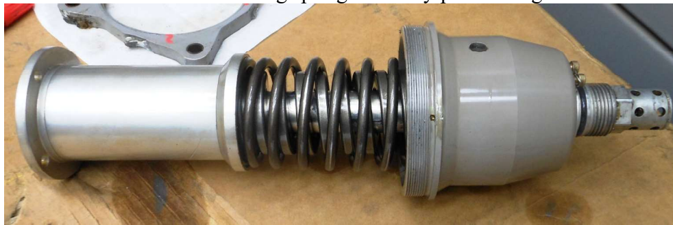
Photo #6 - Feathering spring assembly/pitch change rod
