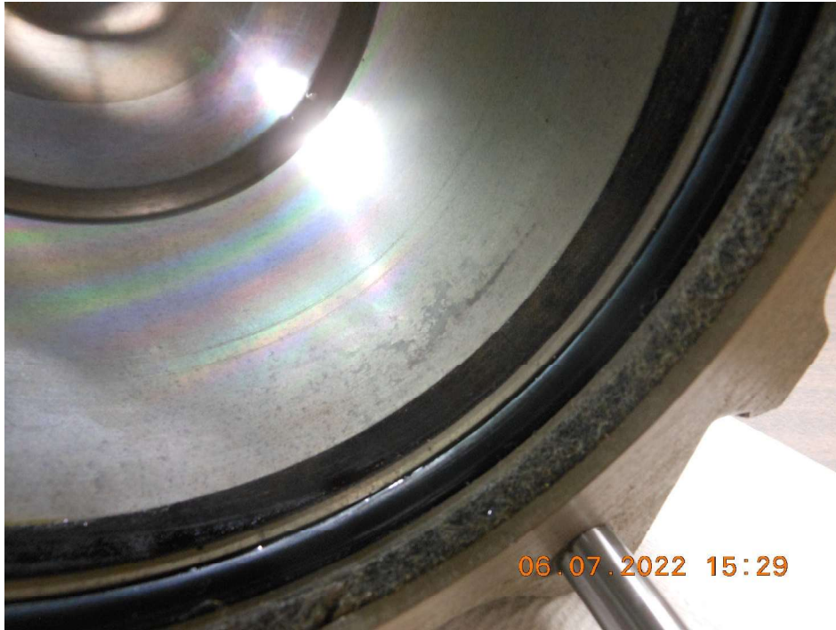
Photo #7 - Piston internal surface marks
