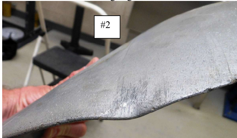
Photo #15 - Blade #2 leading edge bend & chordwise scoring
