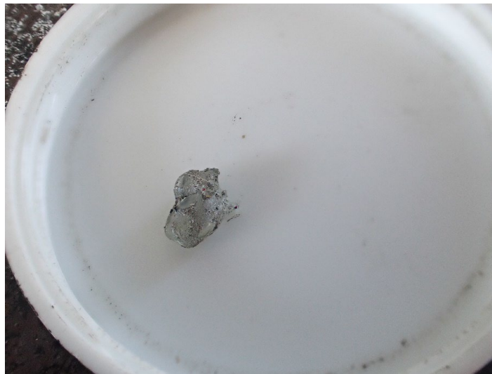
Globule of material removed from fuel strainer, ASI-22-BC-087
