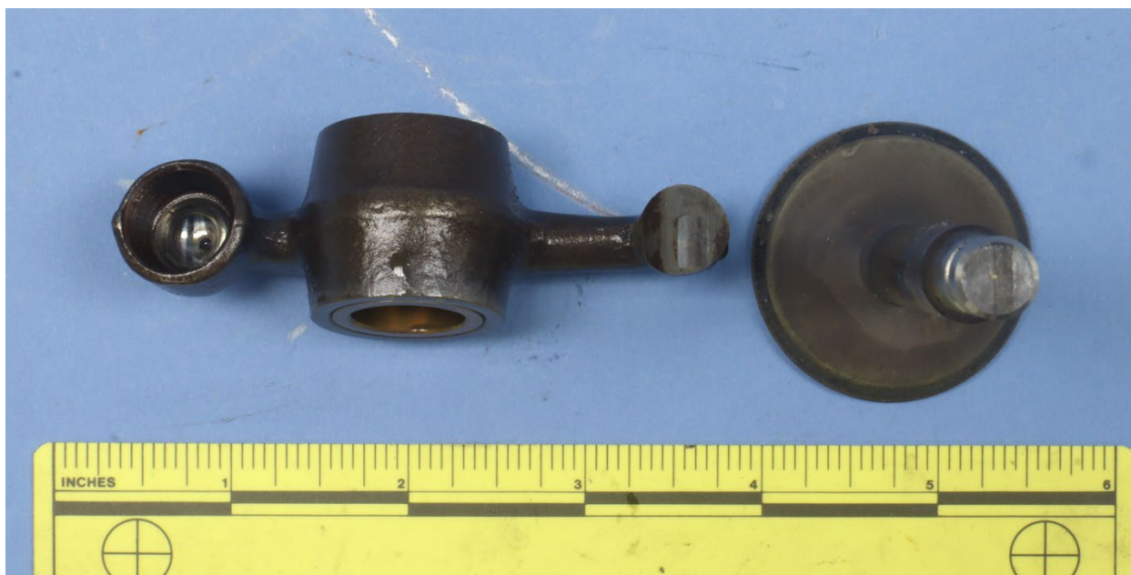
Figure 10. View of the contact surfaces of the rocker arm and exhaust valve stem.
