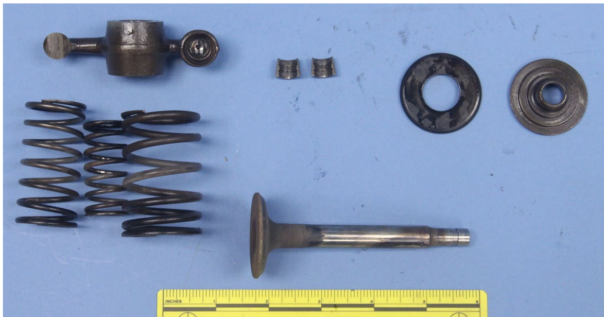
Figure 9. Components from the exhaust side of the #4 cylinder.
