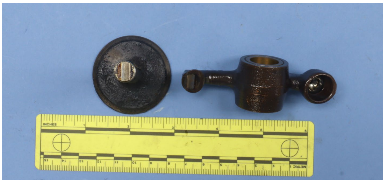
Figure 8. View of the contact surfaces of the rocker arm and intake valve stem.
