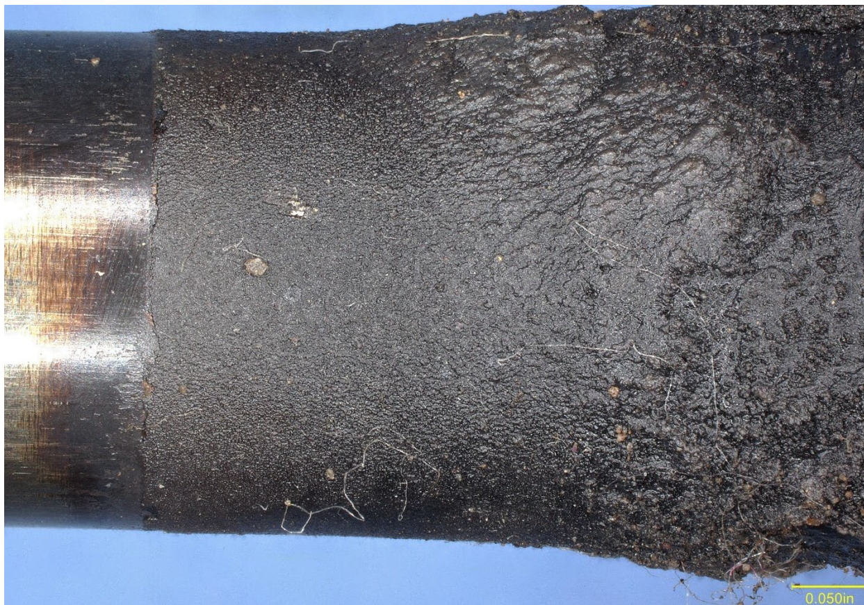
Figure 19. Closer view of the buildup on the stem in Figure 18.
