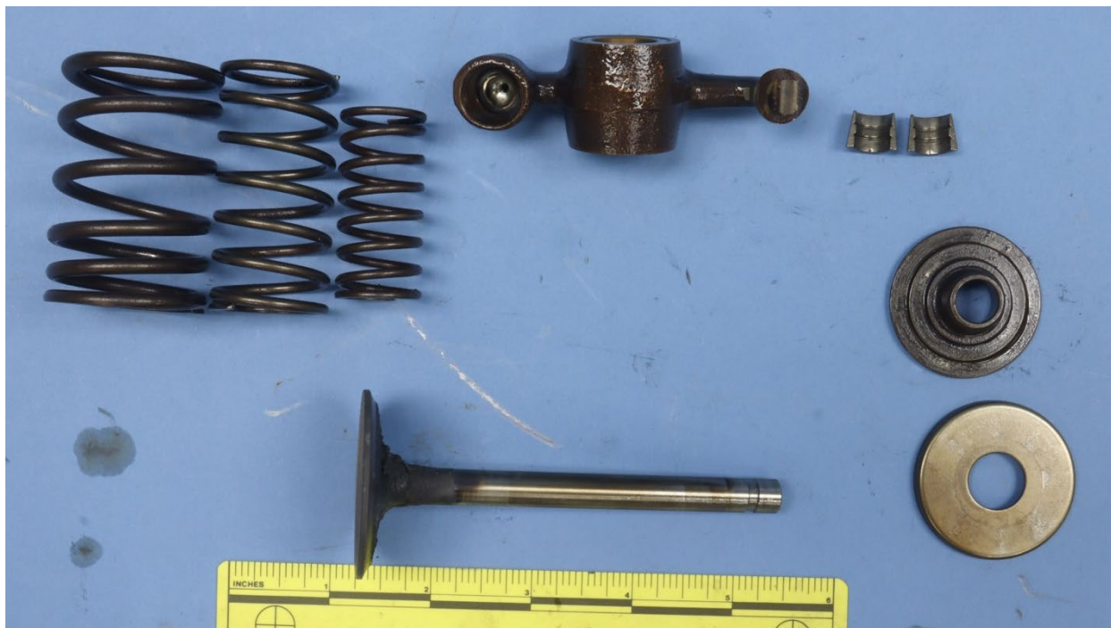
Figure 7. Components from the intake side of the #4 cylinder.
