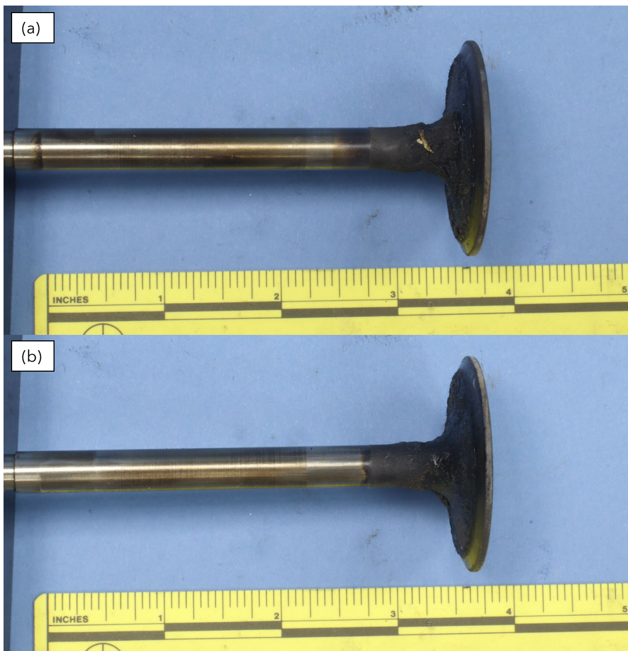
Figure 16. Side views of the stem near the head of the intake valve, rotated 90°.
