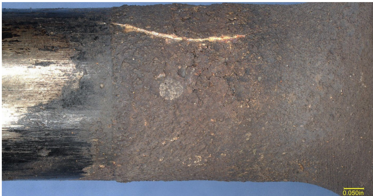
Figure 14. Closer view of the buildup on the stem in Figure 13 .
