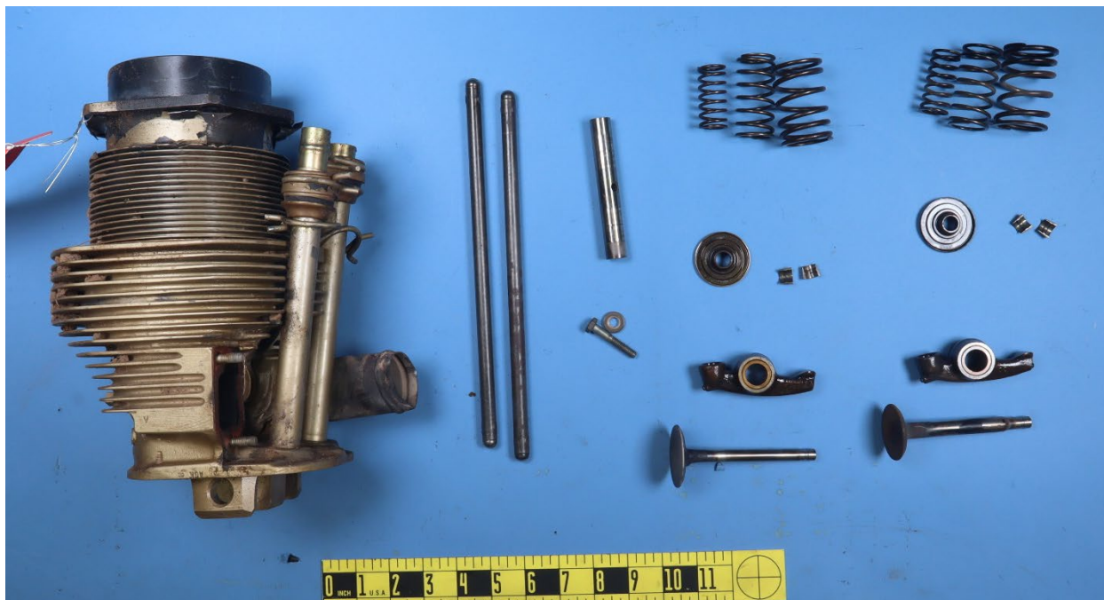
Figure 1. Components from the #4 engine position, as received.
