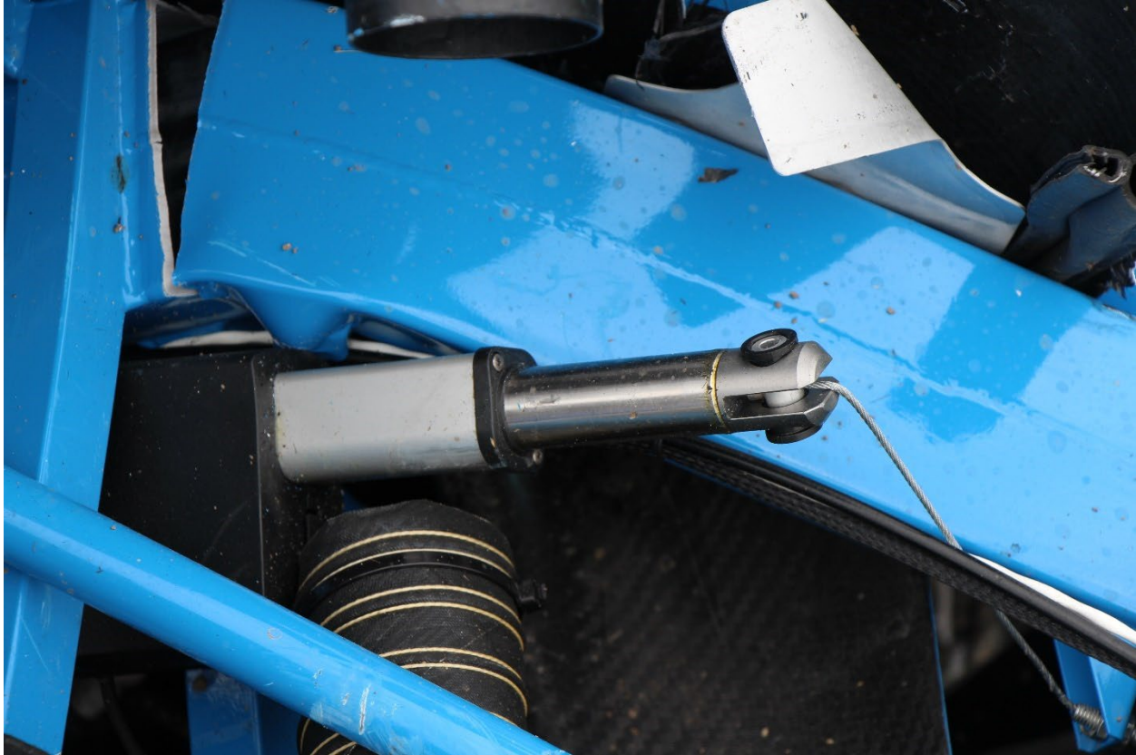
Photograph 6: Electric trim actuator
