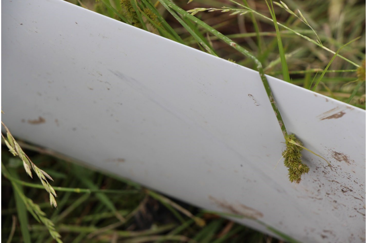
Photograph 4: Black transfer marks on blade 2
