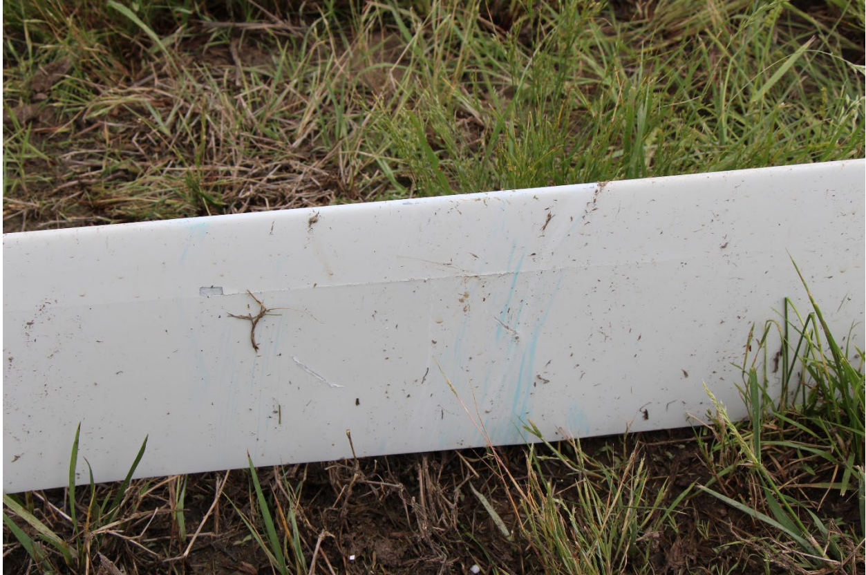
Photograph 5: Blue transfer marks on blade 1
