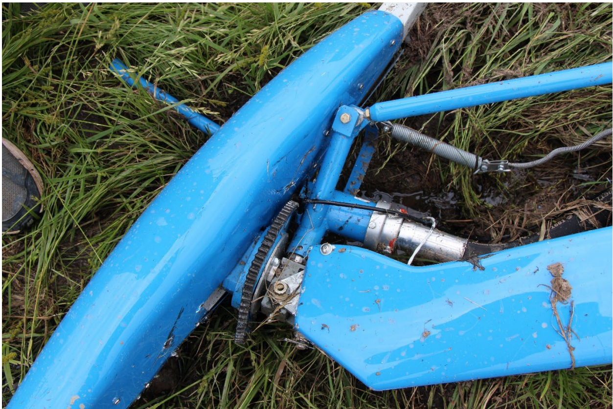
Photograph 3: Bent notched gear and rotor head housing
