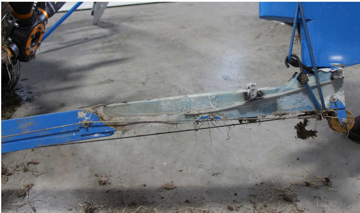
Photograph 3: Left rudder cable hung on main structure bolt
