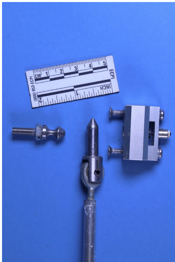
Figure 5. Door pins, closing blocks and locking pins from copilot's side.
