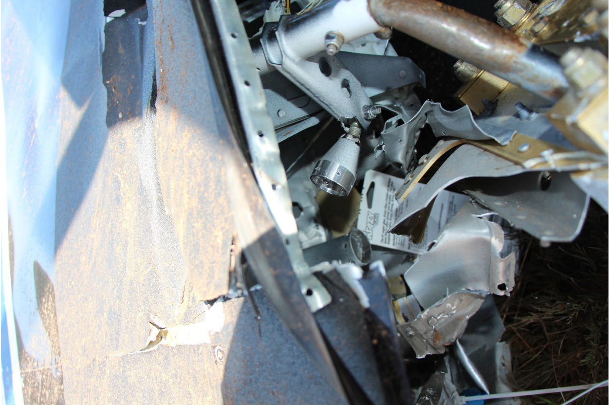
Photograph 5: Right wing torque tube at inboard wing
