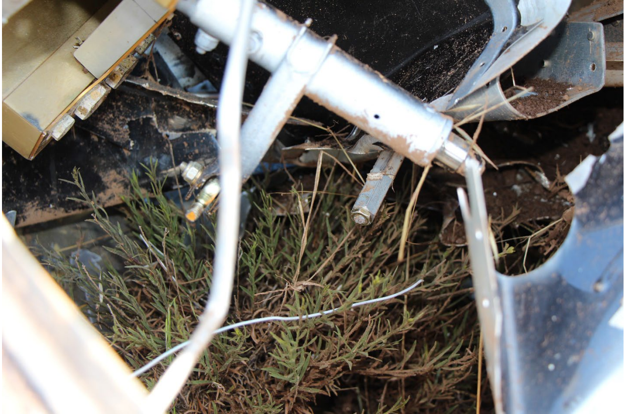
Photograph 6: Fractured rod end and push tube, inboard right aileron
