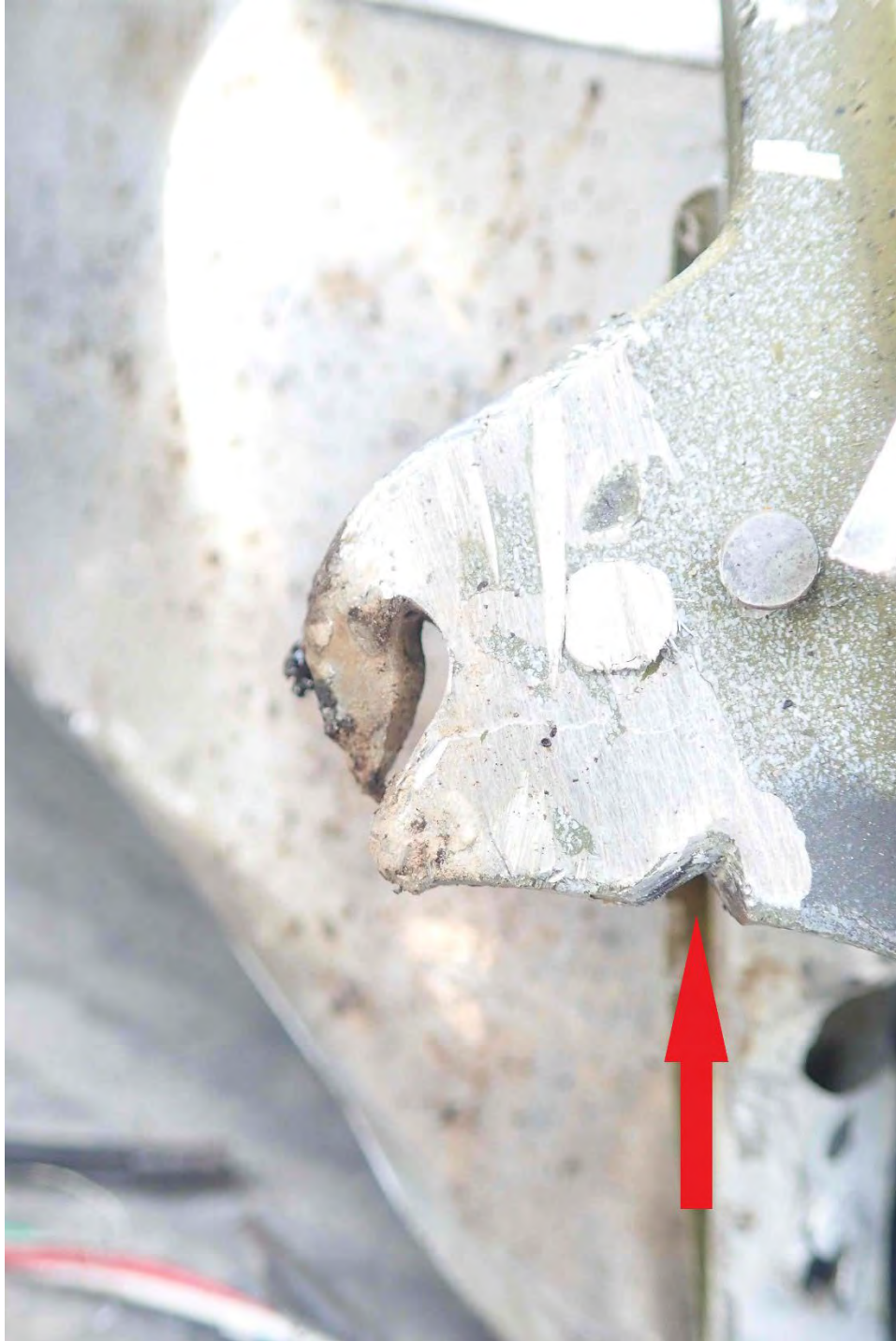
Figure 36 - Aft right wing spar cap notch to upper surface
