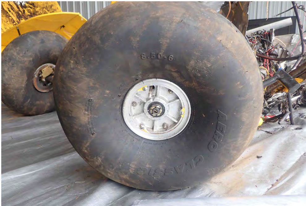
Figure 32 – Right wheel with remnants of yellow hub cap
