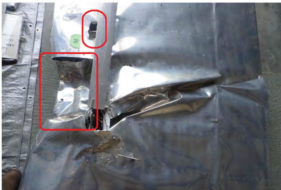
Figure 24 – Right wing outboard lift strut and wheel/step imprints
