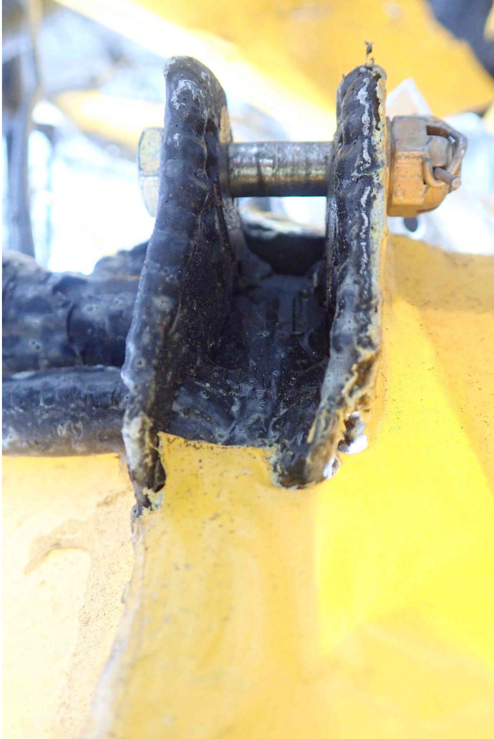
Figure 19 – Rear spar fuselage fitting and bolt
