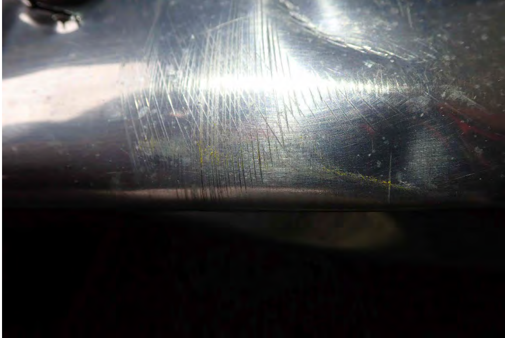
Figure 31 – Yellow transfer mark on right wing indentation
