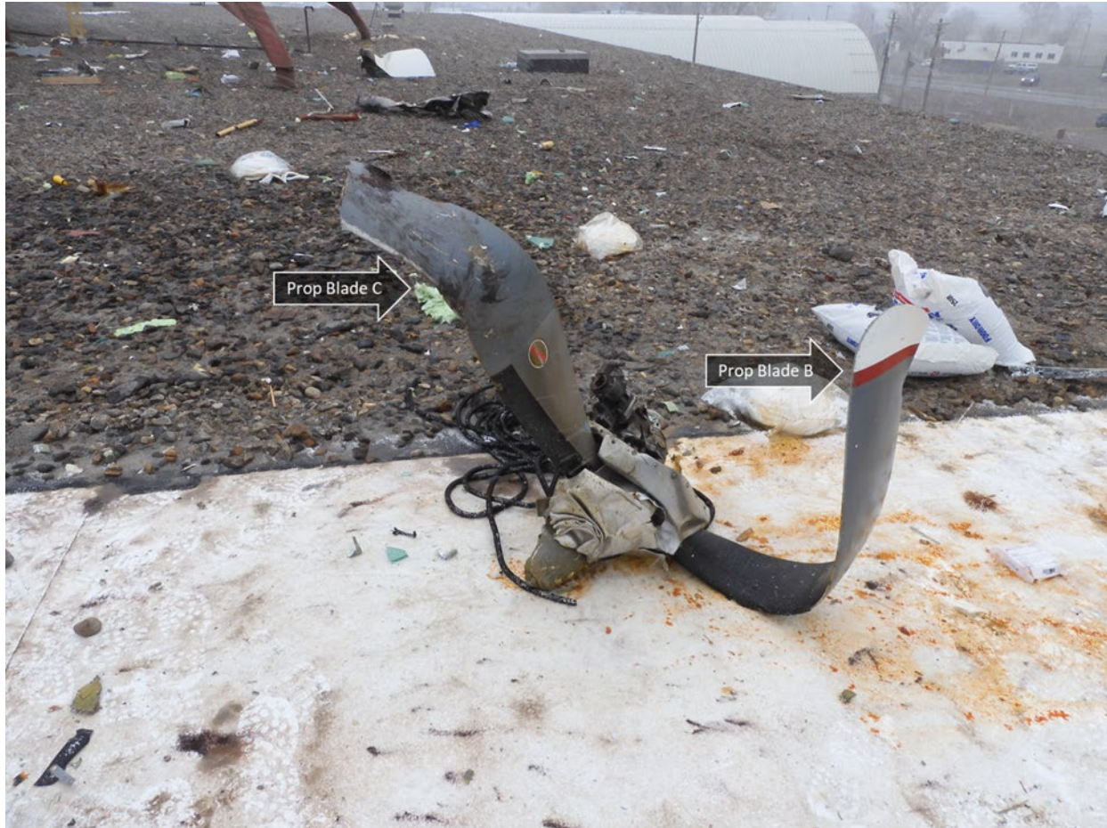
Figure 21. Propeller blade B and C, and propeller hub with spinner.
