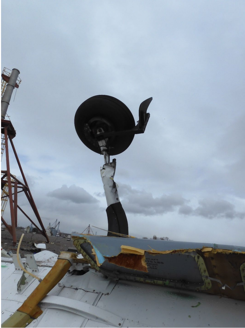
Figure 15. Left-side main landing gear.
