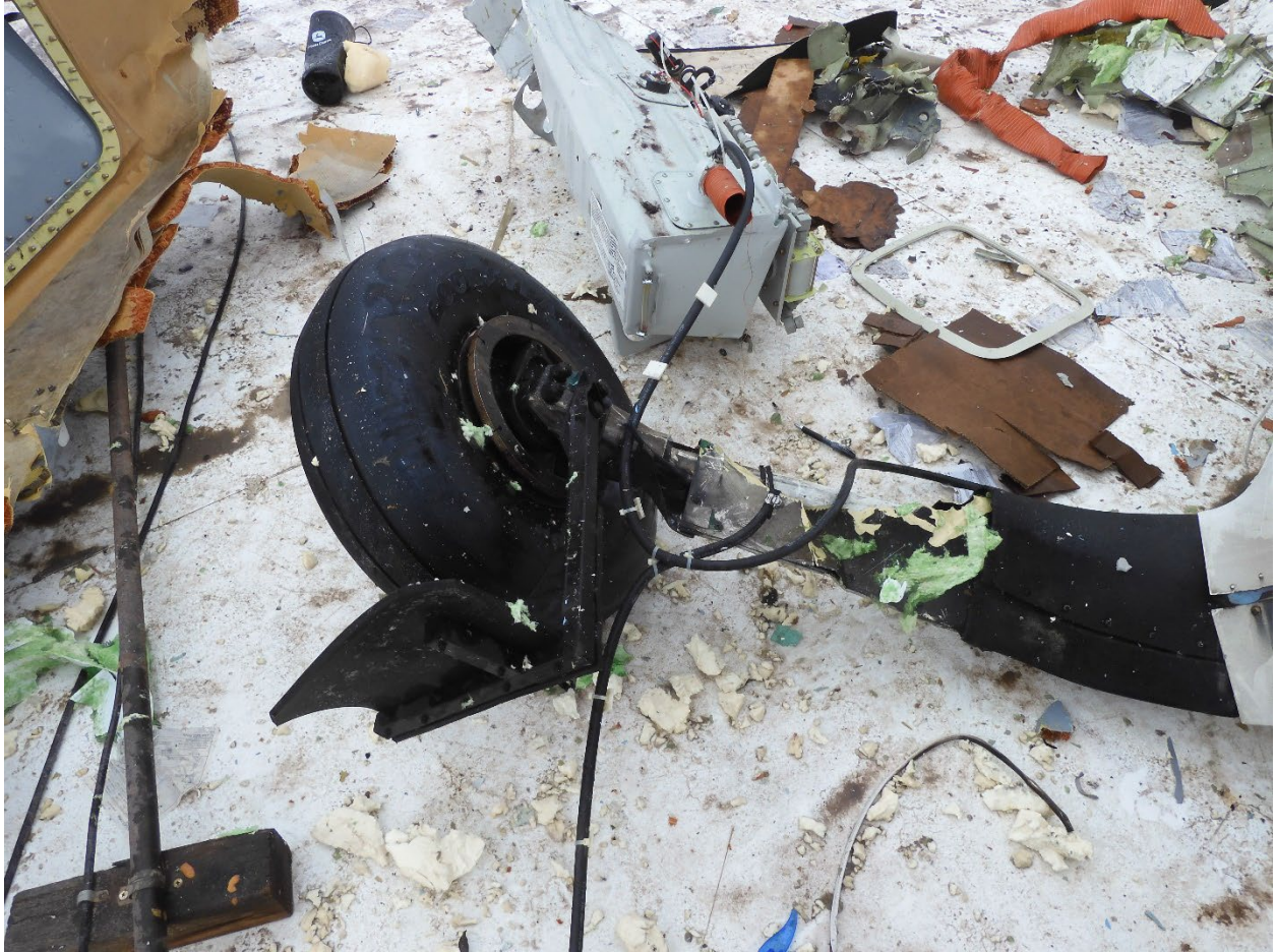
Figure 14. Right-side main landing gear.
