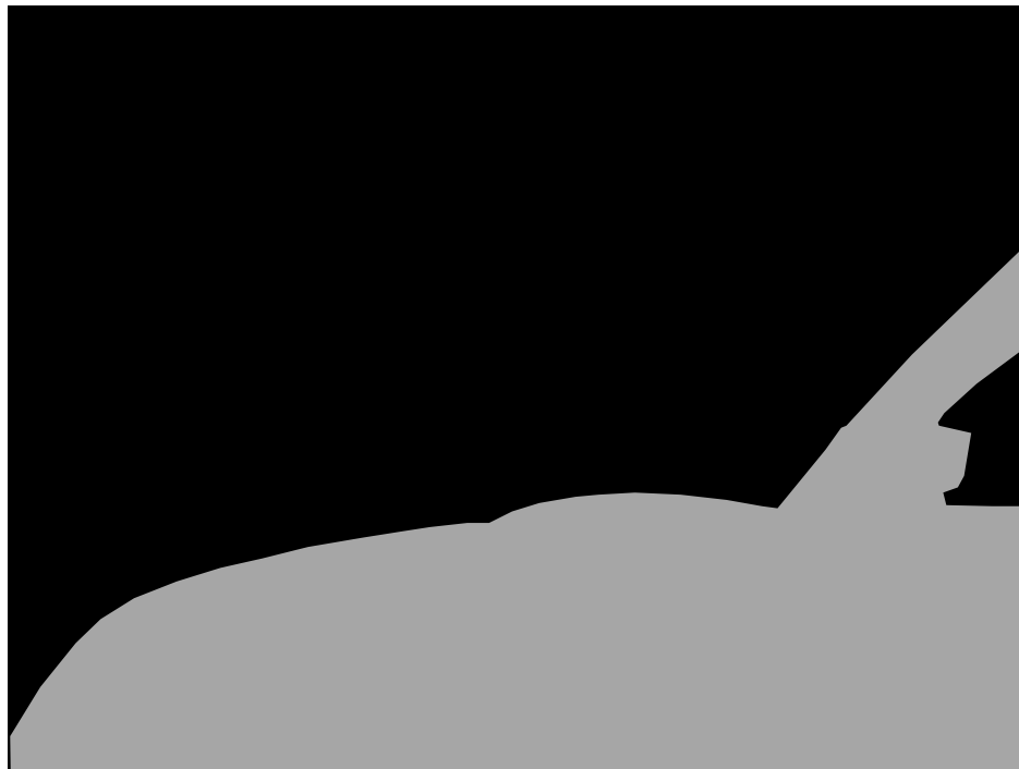
Figure 28b. Instrument panel “mask” for FSX constructed from C208B laser scan data. Black color denotes transparency (windshield); gray color denotes structure (cockpit / cowl).
