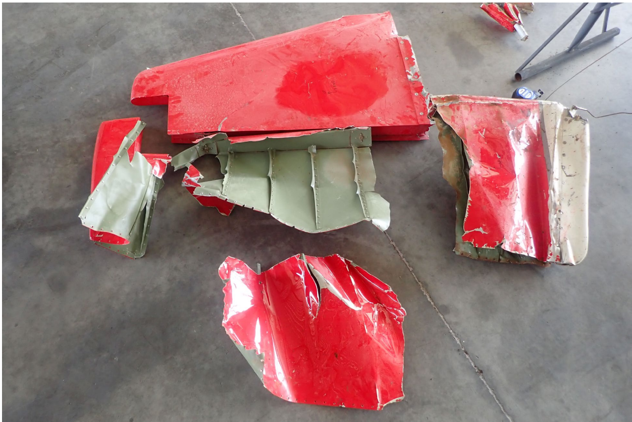
Figure 5. Vertical stabilizer and rudder (NTSB photo).
