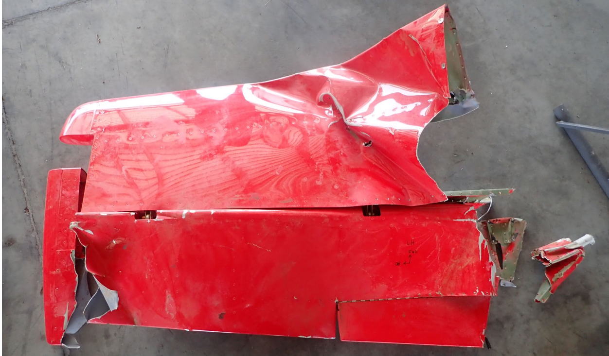
Figure 3. Left horizontal stabilizer and elevator (NTSB photo).
