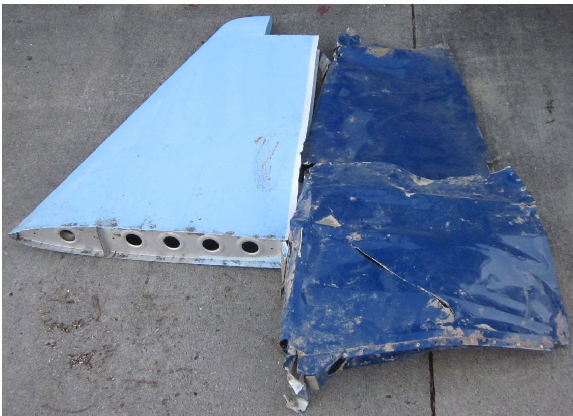
Figure 11. RV-9, N807LK, separated vertical stabilizer and rudder (NTSB photo).
