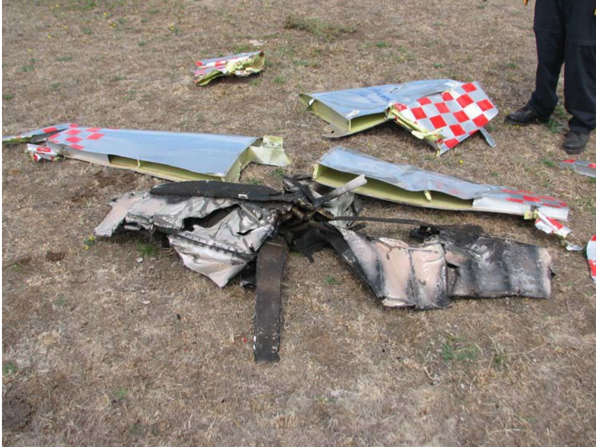
Figure 6. RV-4, VH-ZGH, empennage components layout (ATSB photo).
