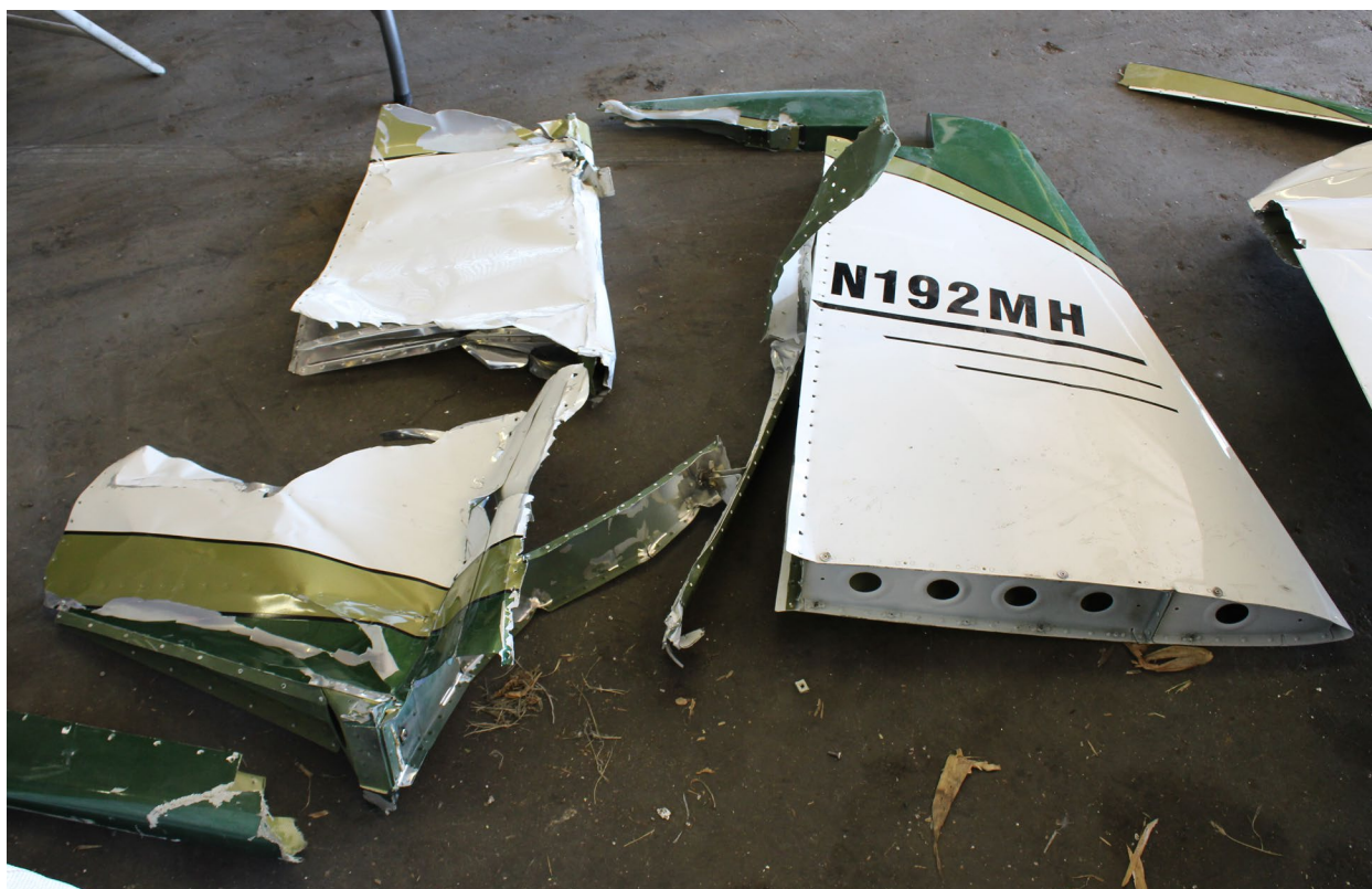
Figure 14. RV-9A, N192MH separated vertical stabilizer and rudder (NTSB photo).
