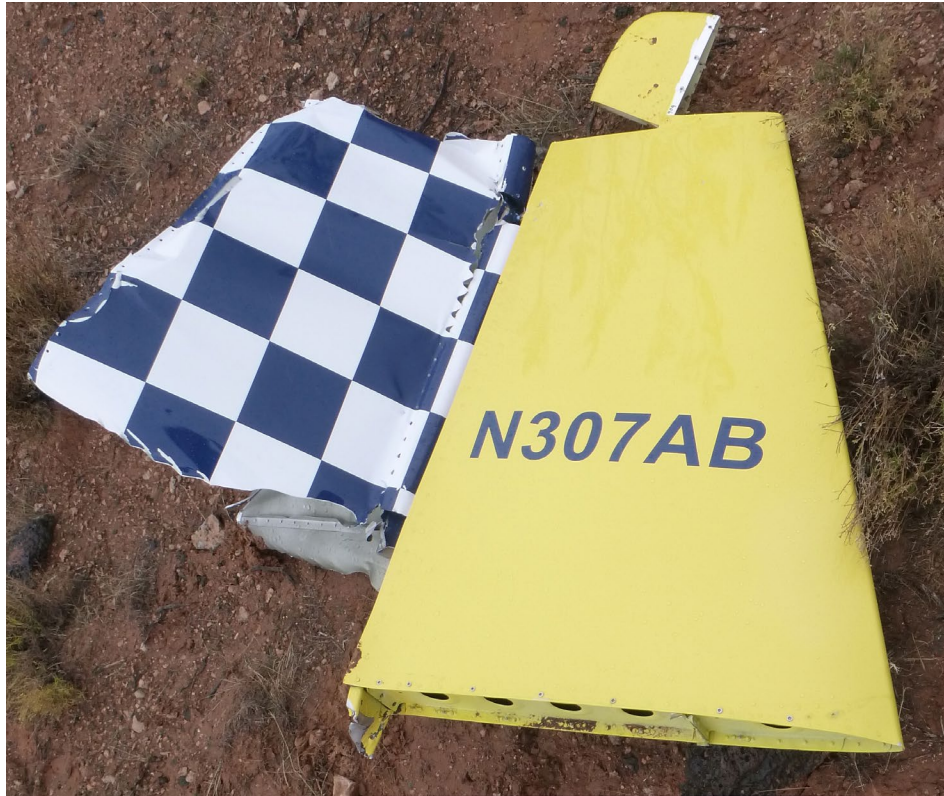
Figure 9. RV-7, N307AB, separated vertical stabilizer and partial rudder (NTSB photo).
