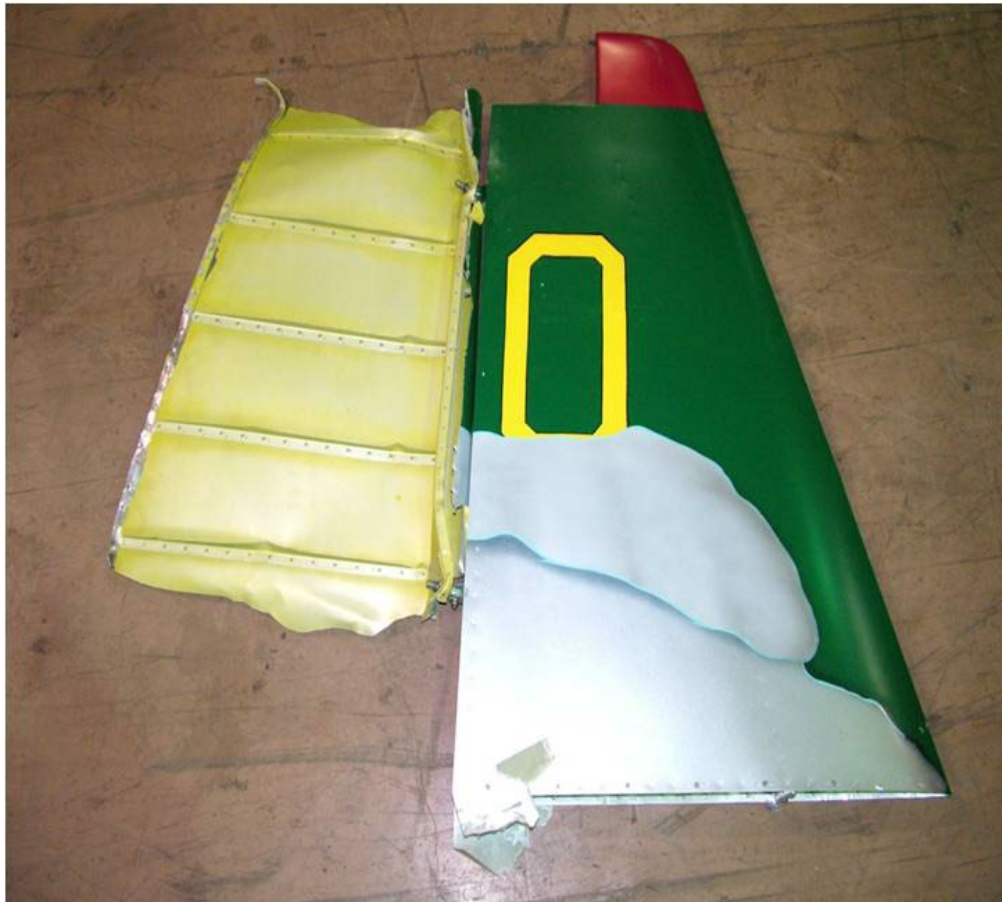
Figure 7. RV-7, G-GNDY, separated vertical stabilizer and rudder (TSB photo).
