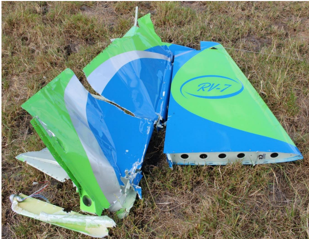
Figure 10. RV-7, ZK-DVS, separated vertical stabilizer and rudder (NZ CAA photo).
