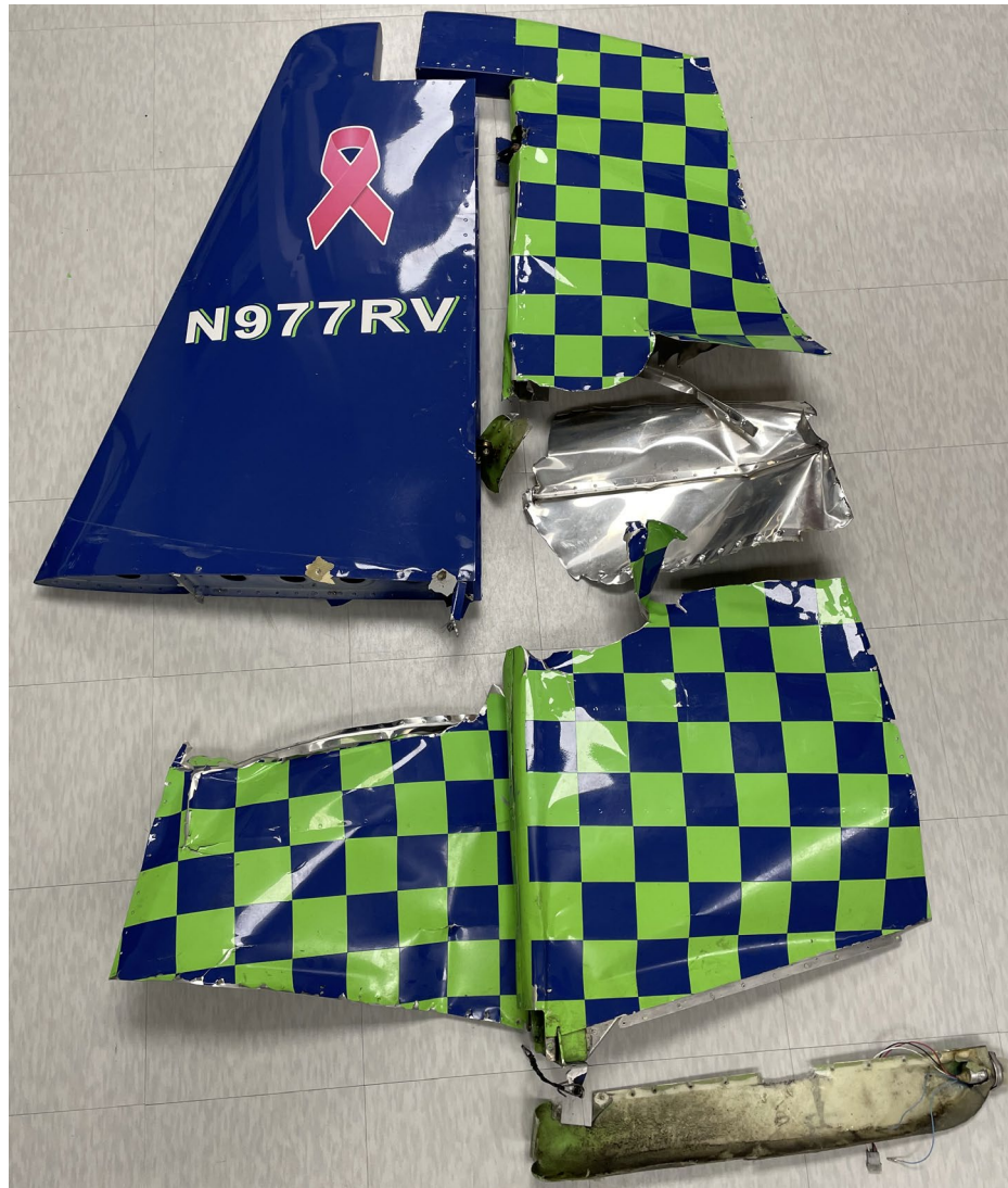
Figure 15. RV-7, N977RV, separated vertical stabilizer and rudder (NTSB photo).
