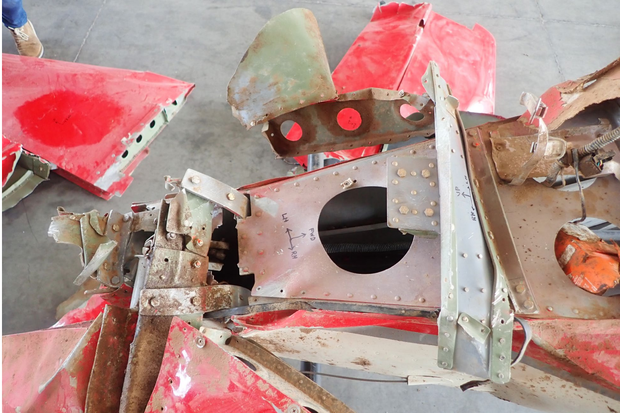
Figure 4. Horizontal and vertical stabilizer attach points, looking down (NTSB photo).
