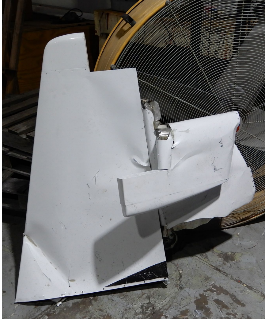
Figure 12. RV-9A, N4889R, separated vertical stabilizer and rudder (NTSB photo).
