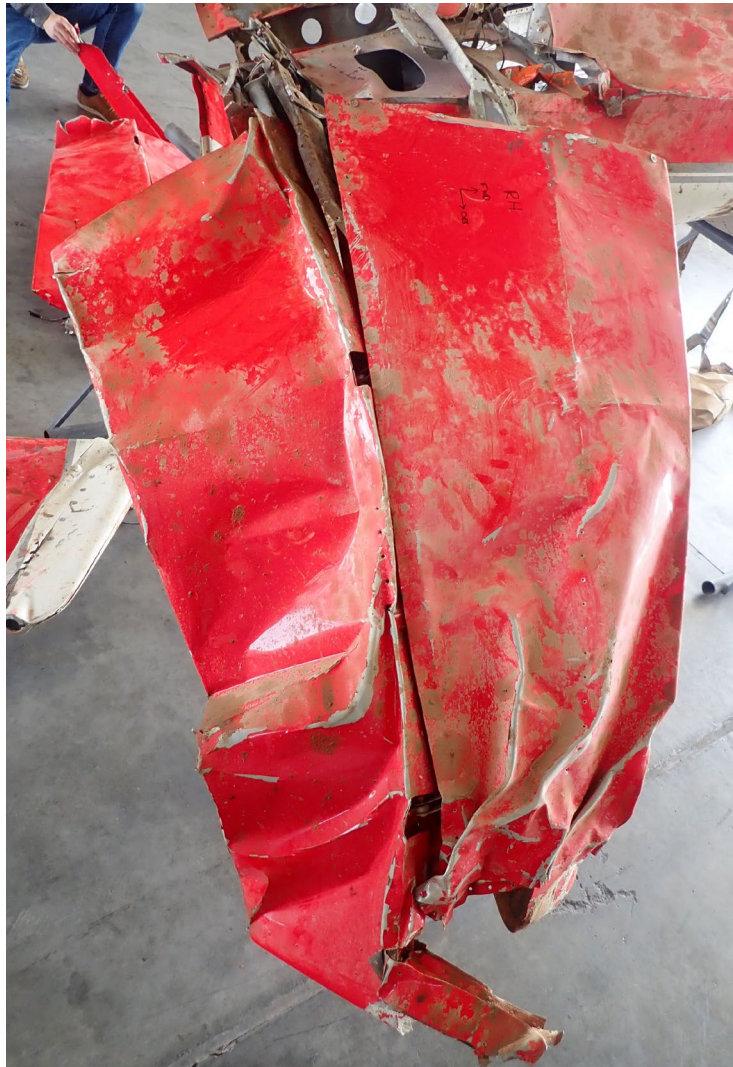
Figure 2. Right horizontal stabilizer and elevator (NTSB photo).
