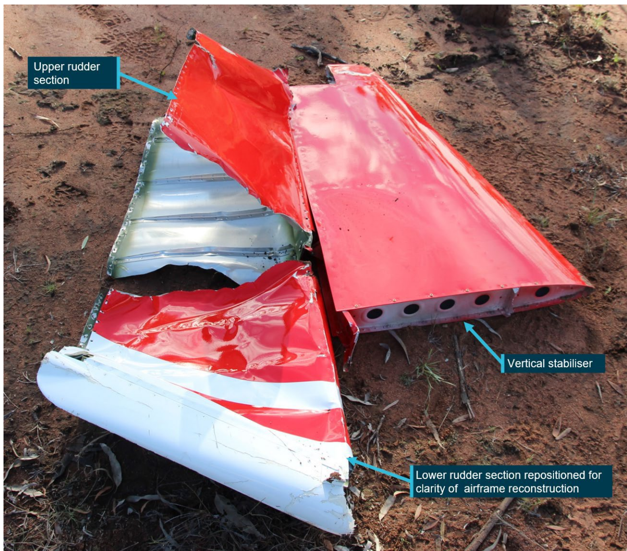
Figure 13. RV-7A, VH-WXI, separated vertical stabilizer and rudder (ATSB photo).
