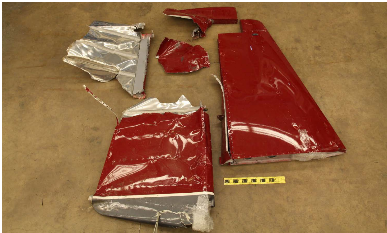
Figure 16. RV-7, N731RV, separated vertical stabilizer and rudder (NTSB photo).
