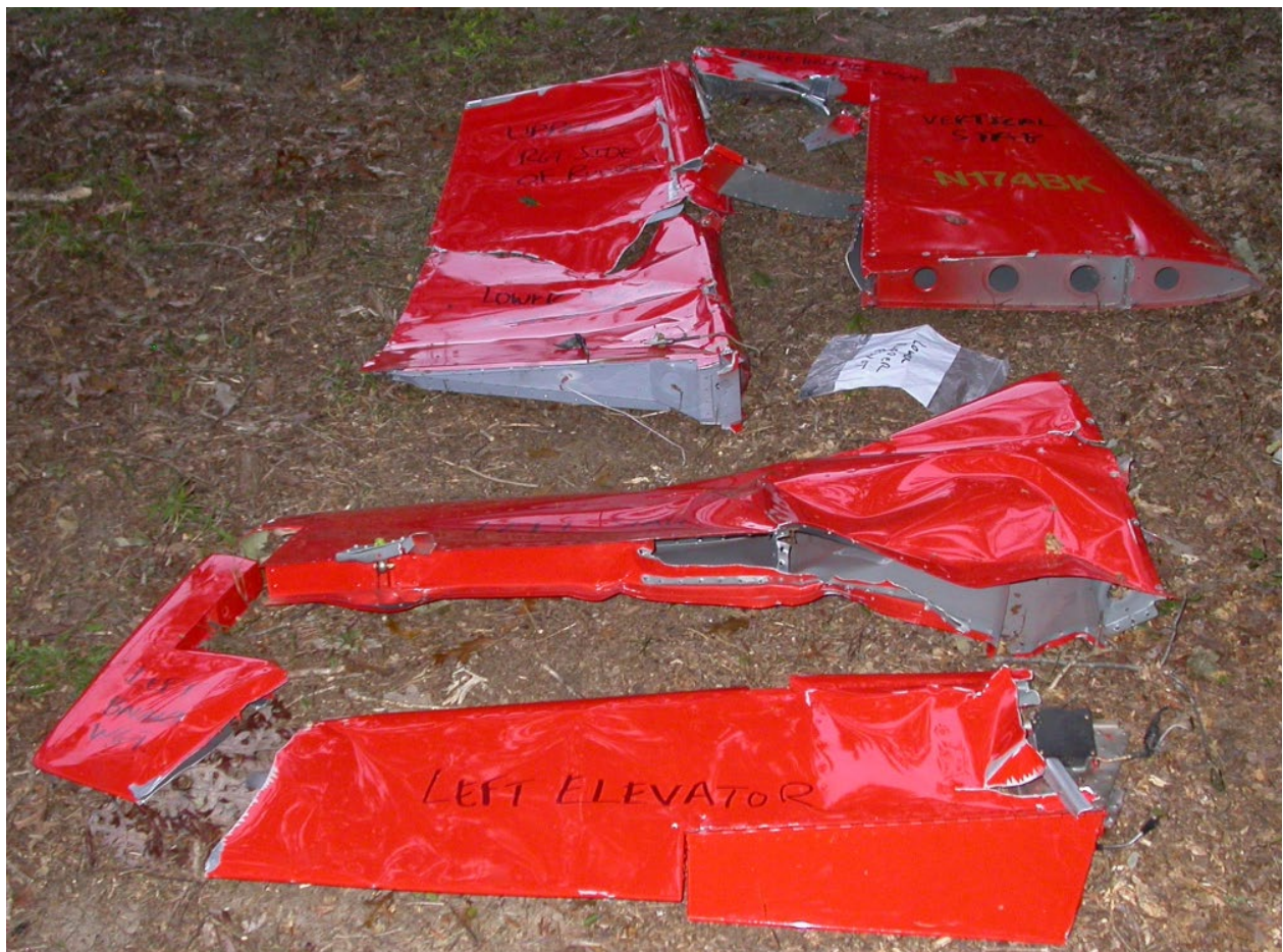
Figure 8. RV-7A, N174BK, separated empennage components (NTSB photo).
