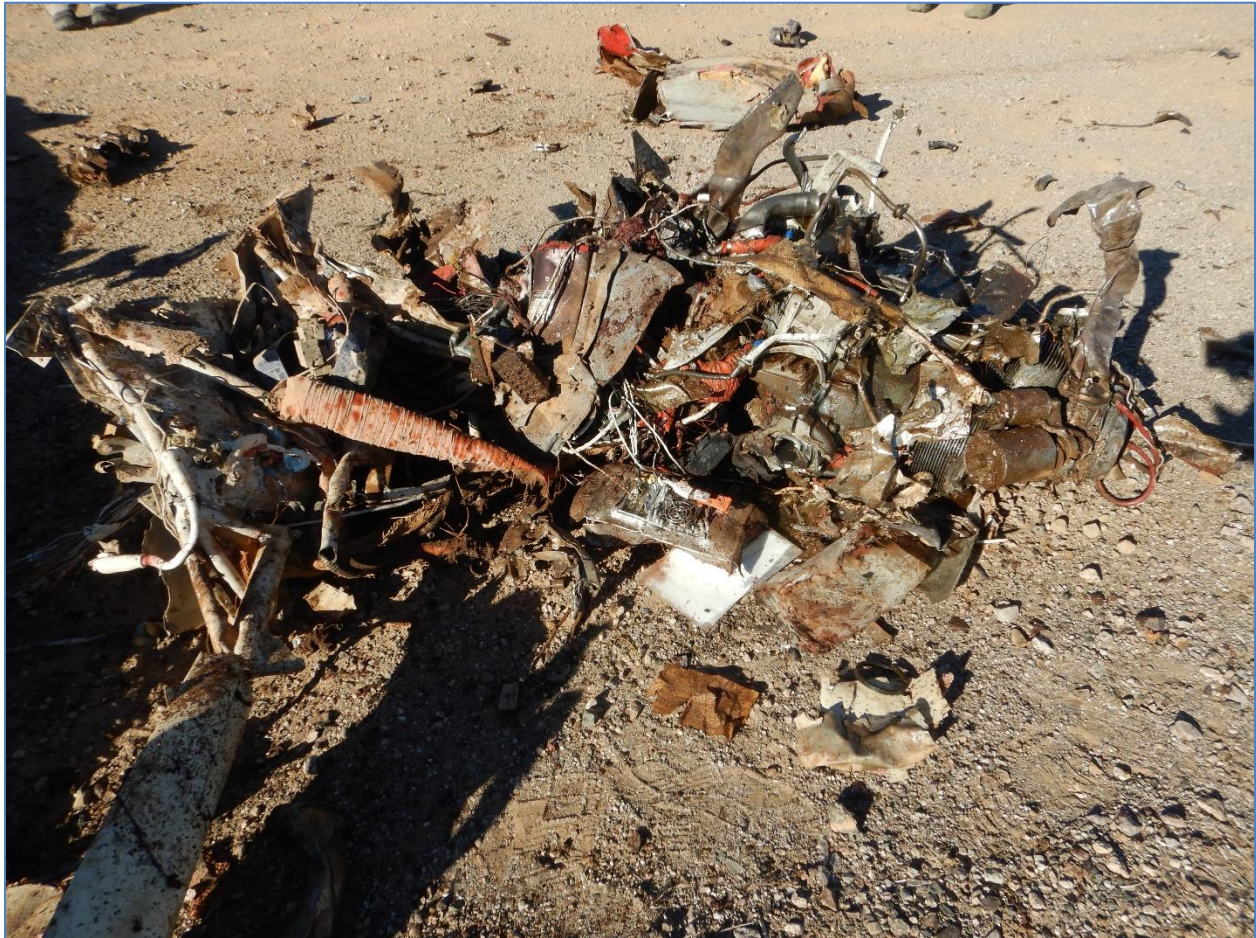
Figure 5-Accident site, right side view of the engine, firewall and engine mounting structure.
