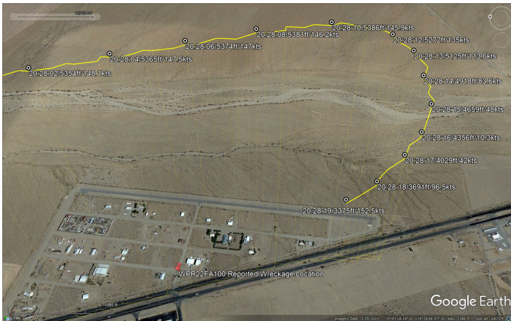
Figure 4. Google Earth overlay showing end of the event flight and reported wreckage location.
