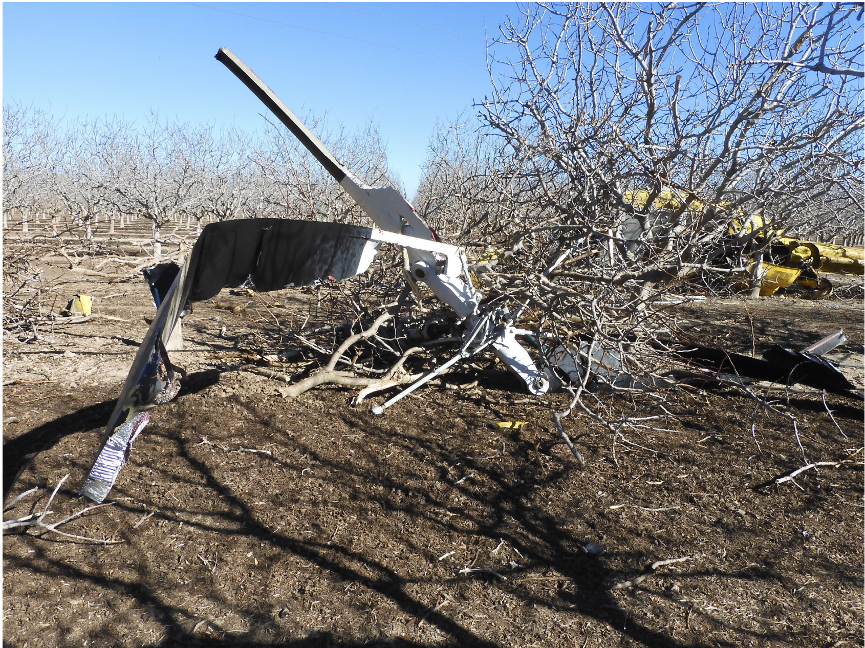
Photo 5 – Main rotor assembly, and transmission.
