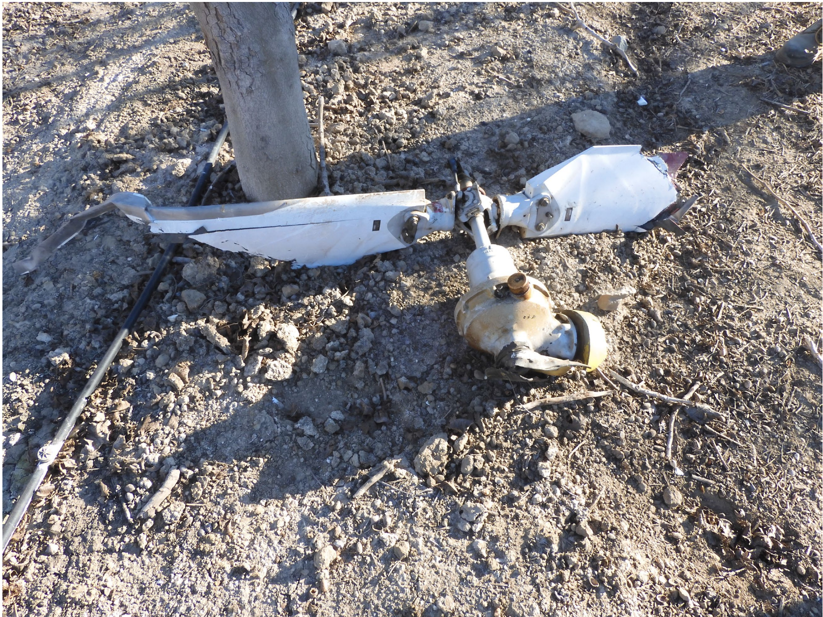
Photo 6 – Tail rotor assembly and 90-degree gearbox.
