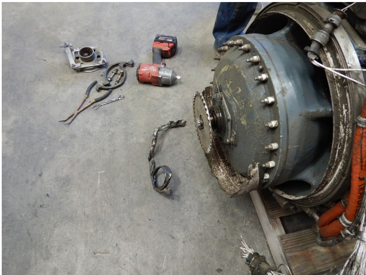
Figure 31. Front of engine with a piece of fire wall removed from around the output shaft.
