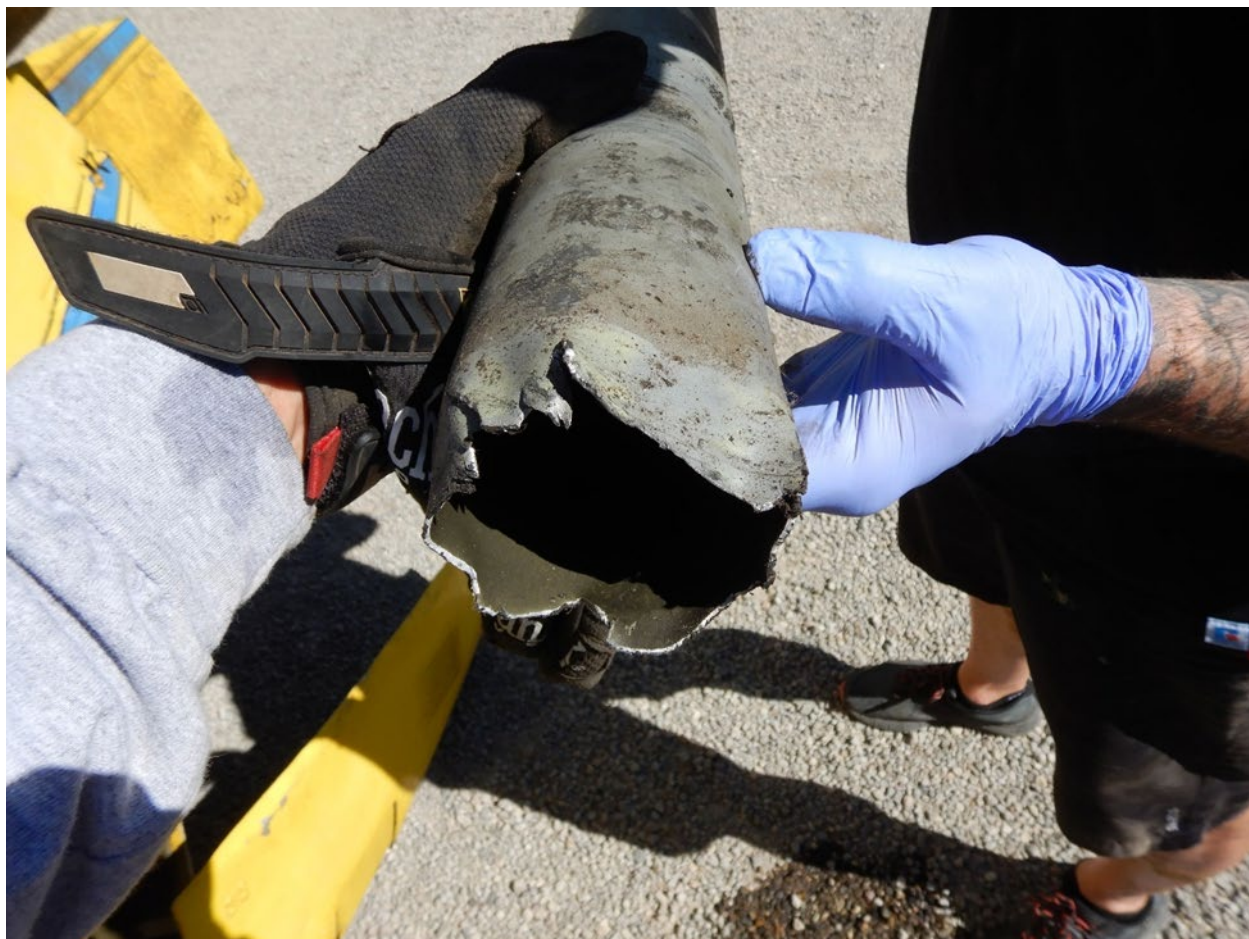
Figure 24. Tail rotor drive shaft that was connected to the transmission output quill. See photo 23.
