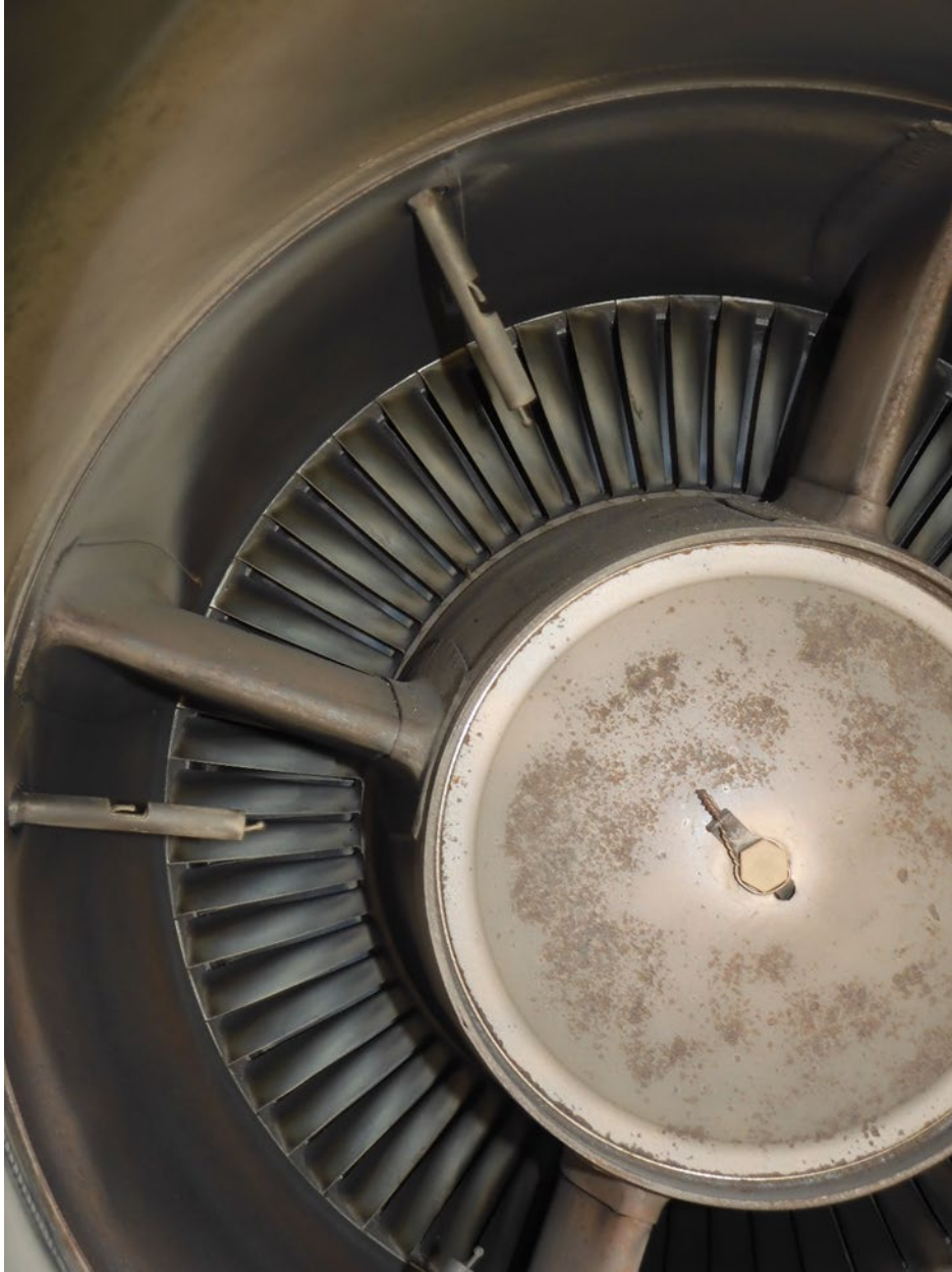
Figure 34. Rear view of engine, showing no damage to the 4th stage turbine wheel.
