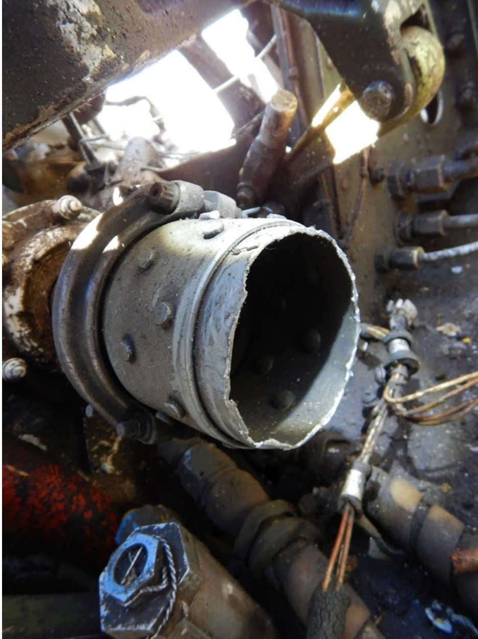
Figure 23. Tail rotor drive shaft, at the transmission output quill.
