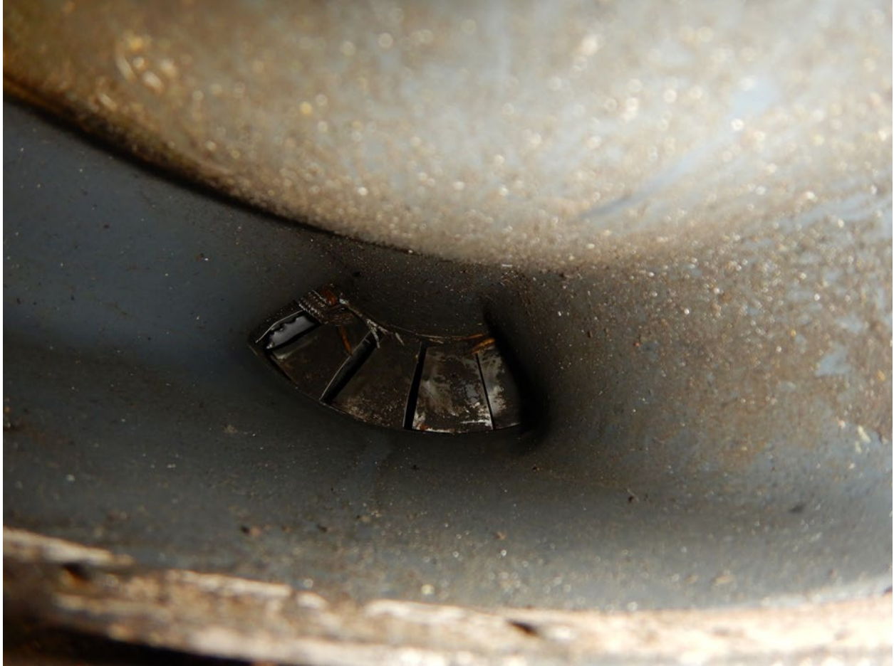
Figure 33. Engine inlet showing damage to a 1st stage compressor blade and the variable inlet guide vanes.
