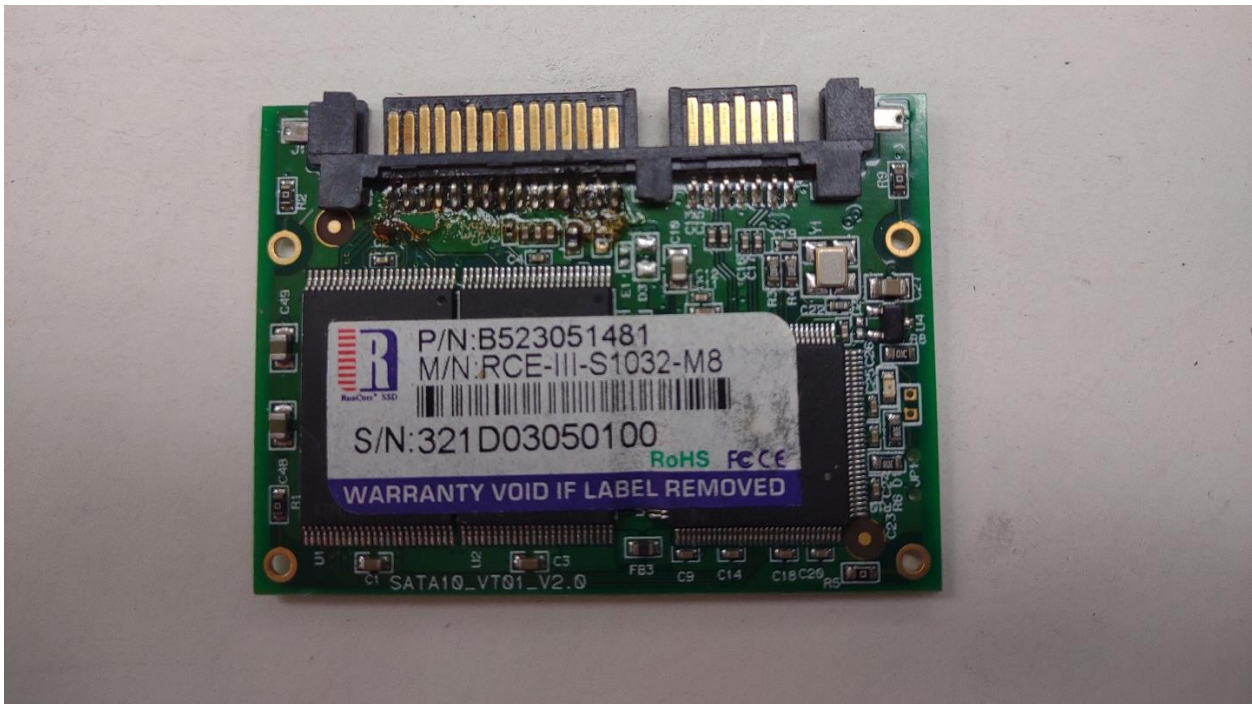
Figure 2. SSD Memory Module removed from the Satloc G4 CPU Module
