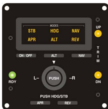
Fig. 2-12. AP Display, TRIM UP Lamp Re-illuminated (System Fifty)
