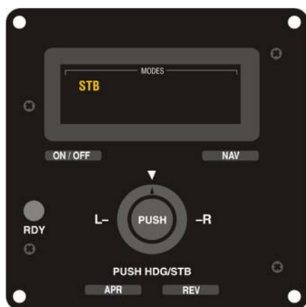
Fig. 2-5. AP Display, STB Mode Engaged (System Forty)
