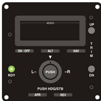
Fig. 2-15. AP Display, RDY for Operation (System Fifty)
