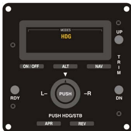
Fig. 2-18. AP Display, HDG Mode Engaged (System Fifty)
