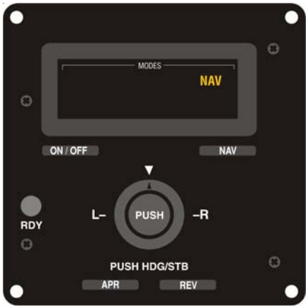
Fig. 2-7. AP Display, NAV Mode Engaged (System Forty)
