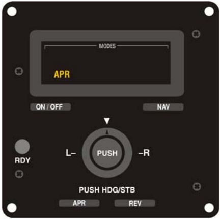
Fig. 2-8. AP Display, APR Mode Engaged (System Forty)
