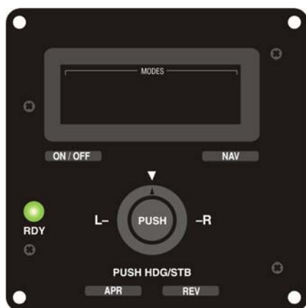
Fig. 2-3. AP Display, RDY for Operation (System Forty)
