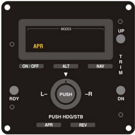
Fig. 2-20. AP Display, APR Mode Engaged (System Fifty)
