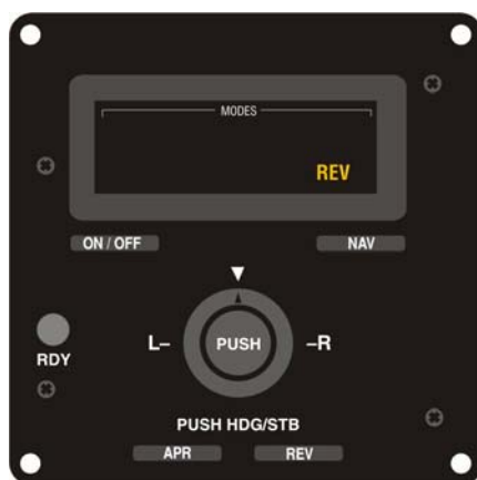
Fig. 2-9. AP Display, REV Mode Engaged (System Forty)
