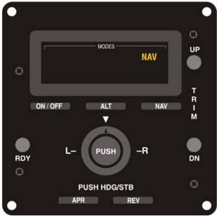
Fig. 2-19. AP Display, NAV Mode Engaged (System Fifty)
