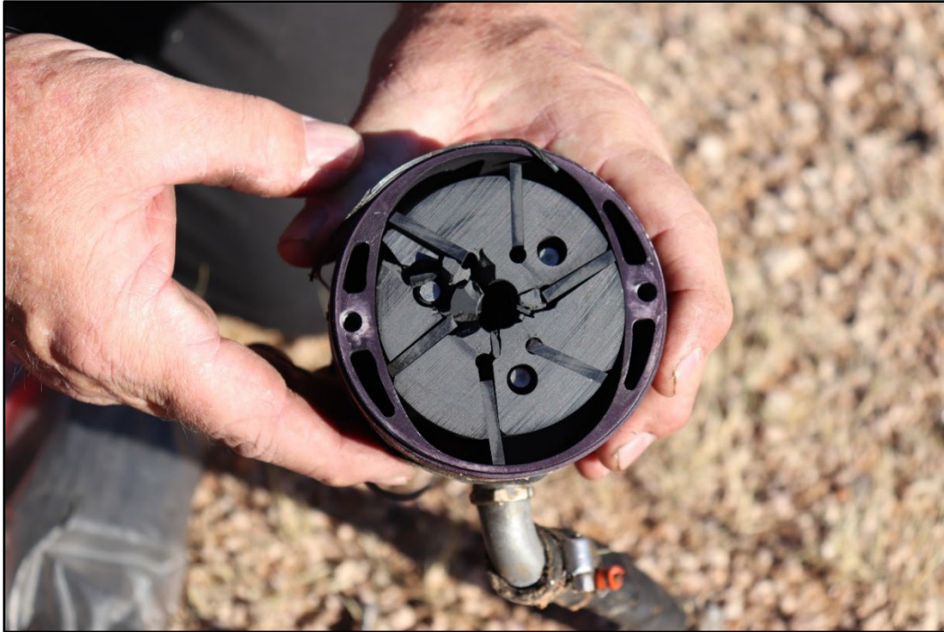
Figure 12: View of vacuum pump.
