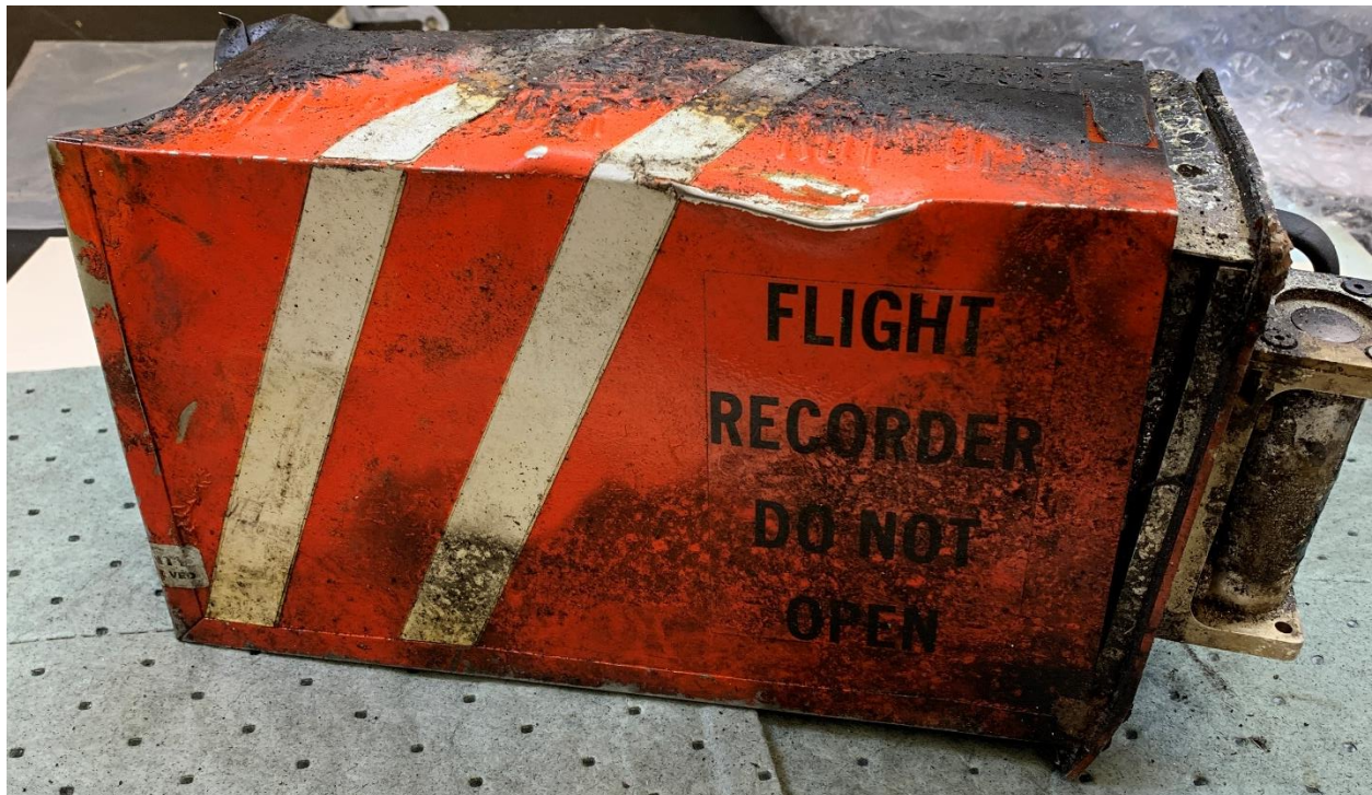
Figure 1. The CVR exterior, as received in the lab, showing thermal and structural damage.
