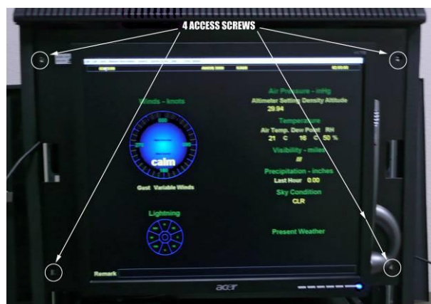
Figure 6. Four Screws Securing Top Shelf
