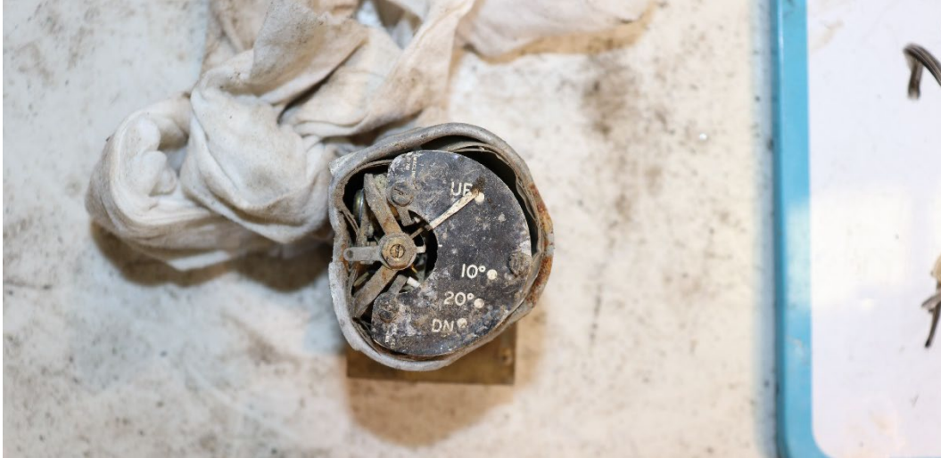
Figure 7: View of flap position indicator. (Photo courtesy of the NTSB)
