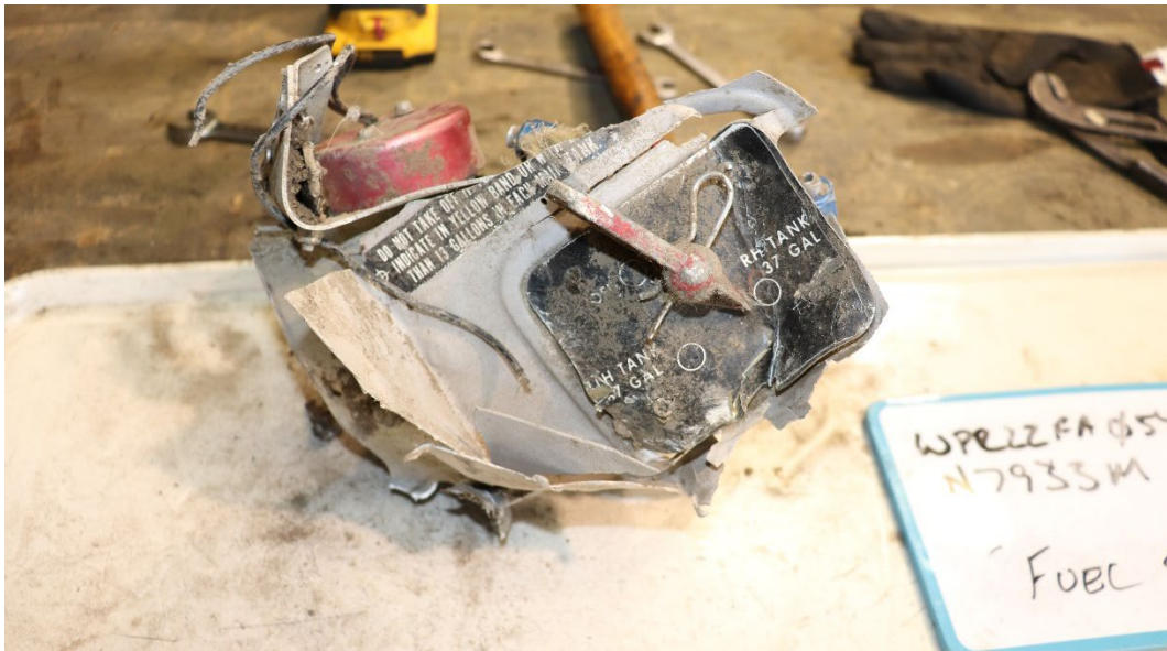
Figure 9: View of fuel selector lever in the right tank position. (Photo courtesy of the NTSB)
