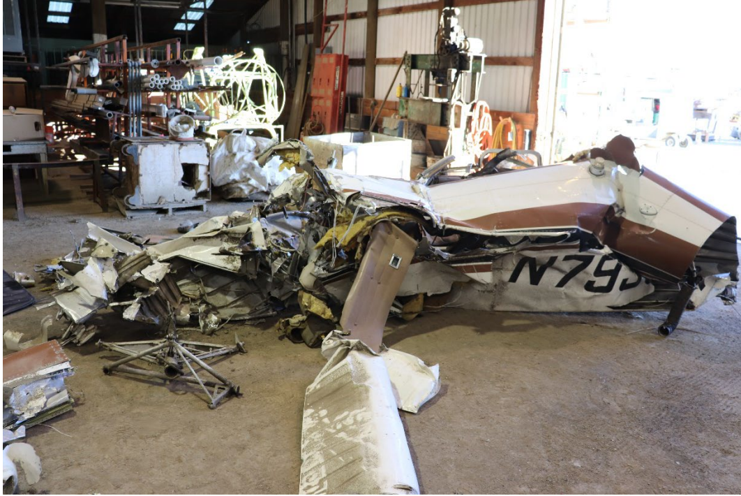
Figure 1: View of airplane cockpit area with impact damage. (Photo courtesy of NTSB)
