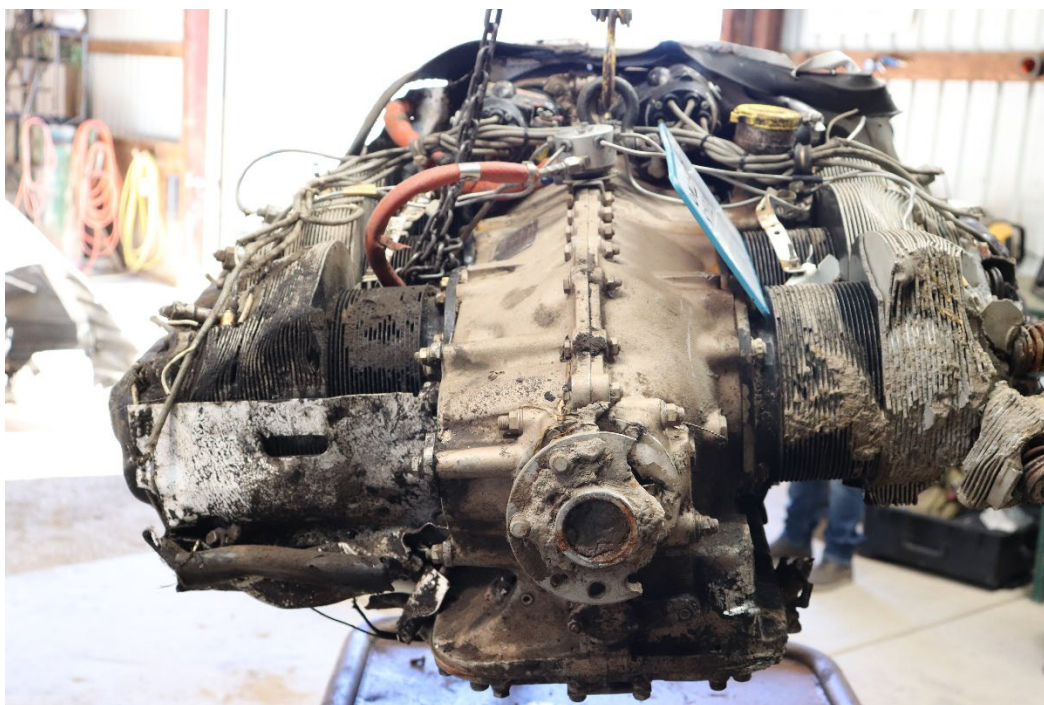
Figure 10: Front view of engine with impact damage. (Photo courtesy of the NTSB)
