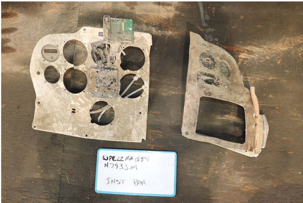
Figure 2: View of airplane instrument panel with various instruments separated. (Photo courtesy of the NTSB)
