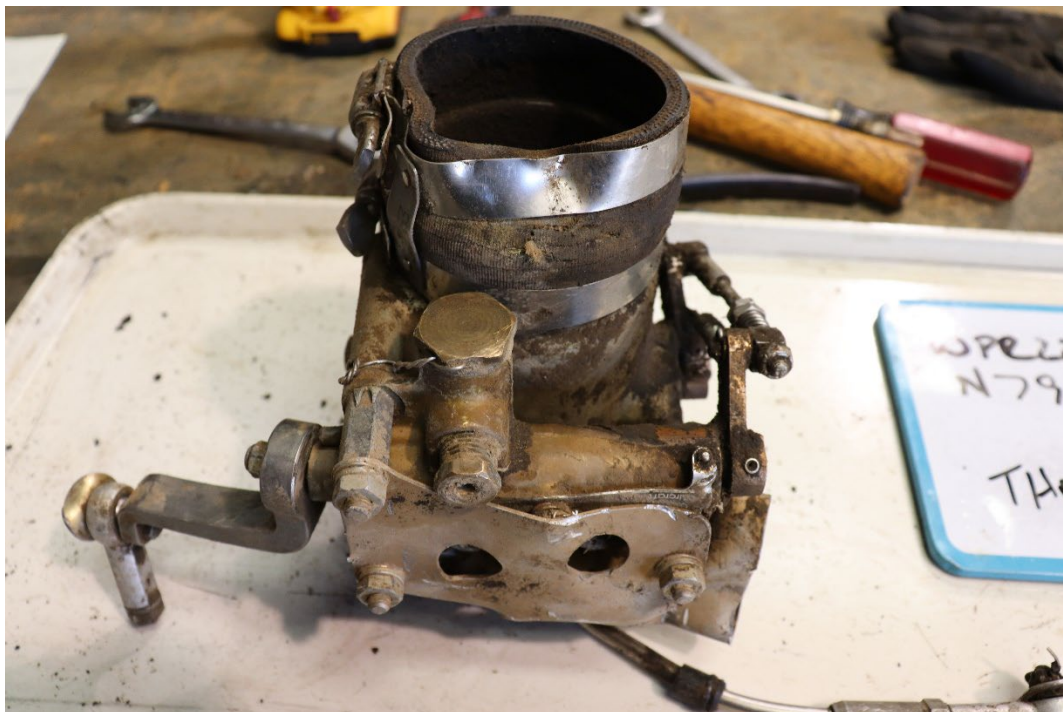
Figure 14: View of throttle body with impact damage. (Photo courtesy of the NTSB)
