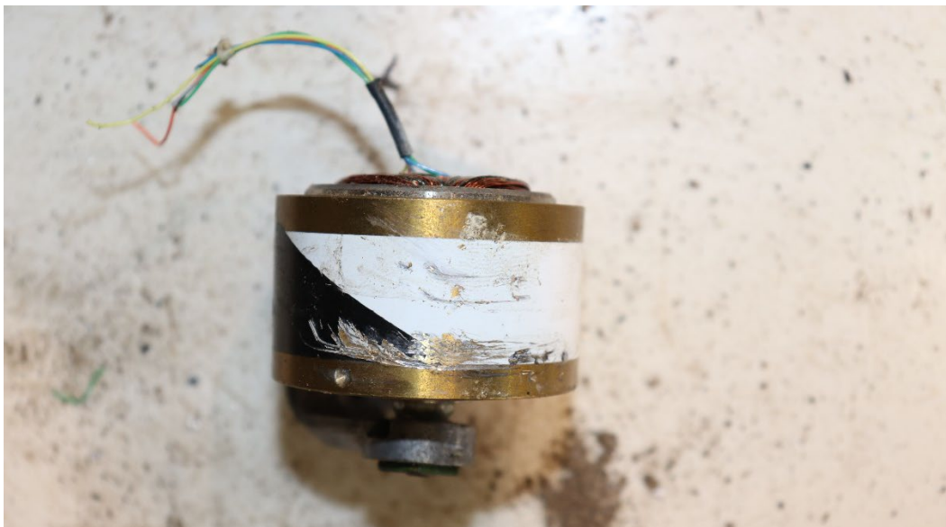
Figure 4: View of unknown instrument gyro gimble with rotational scoring and impact damage. (Photo courtesy of the NTSB)
