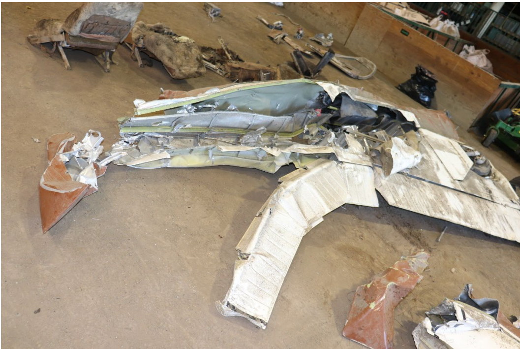
Figure 6: View of right wing with impact damage. (Photo courtesy of the NTSB)
