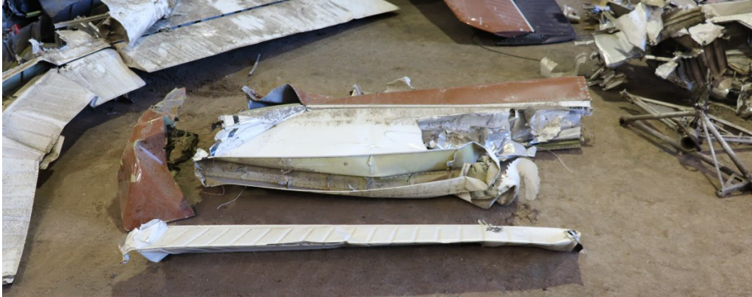
Figure 5: View of left wing with impact damage. (Photo courtesy of the NTSB)
