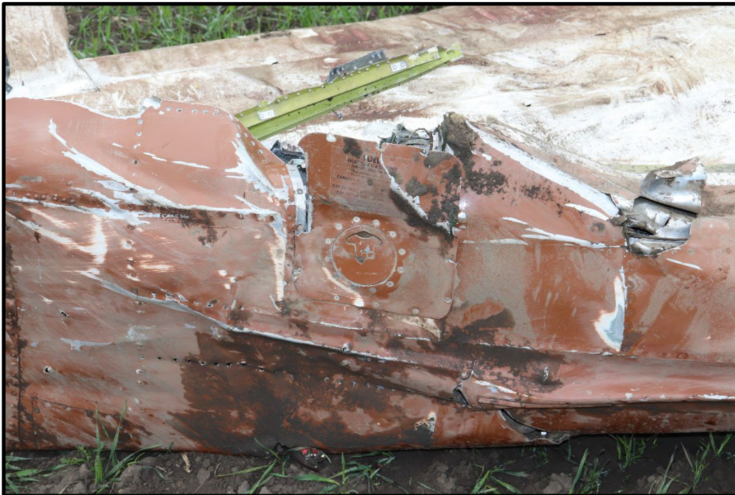
Figure 9: View of right main fuel tank cap (photo courtesy of the NTSB)
