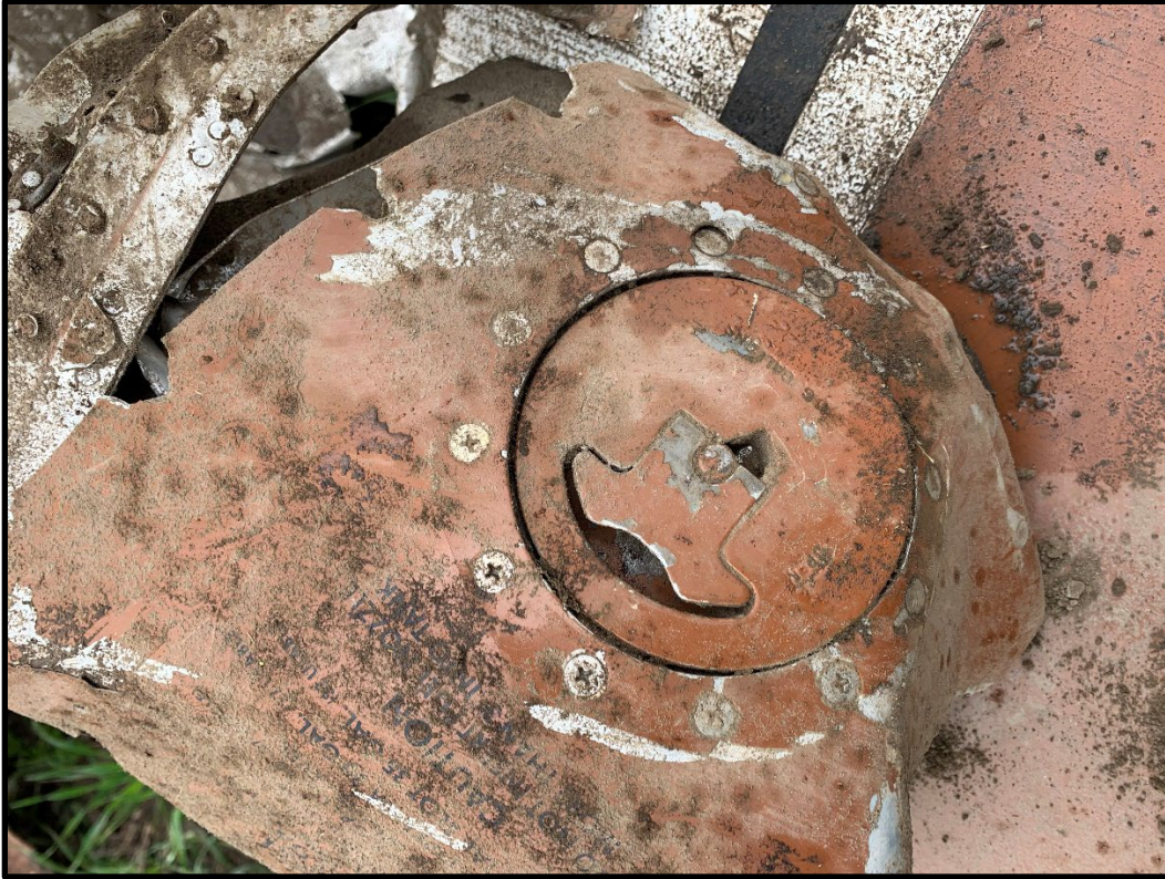
Figure 7: View of left main fuel tank cap (photo courtesy of the NTSB)
