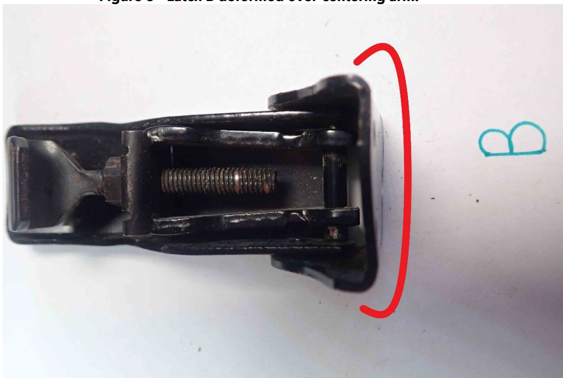
Figure 7 - Latch B twisted mounting plate.
