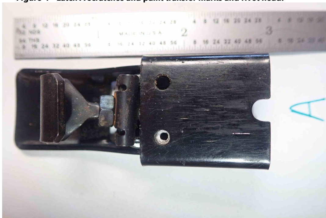
Figure 5 - Latch A mating side of the mounting plate scratches and grooves in the vertical plane.
