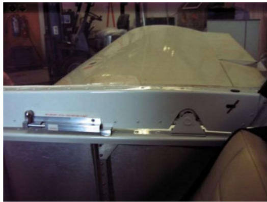
Figure 2 above: a simple barrel latch fitted on both sides of the canopy.
