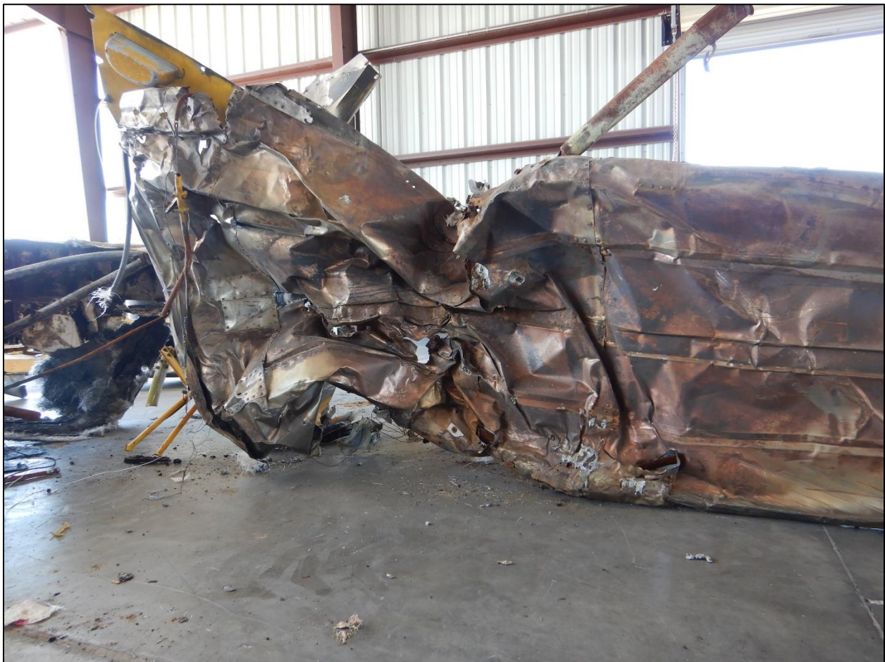
Figure 5-Impact signature on cabin area, lower pan.
