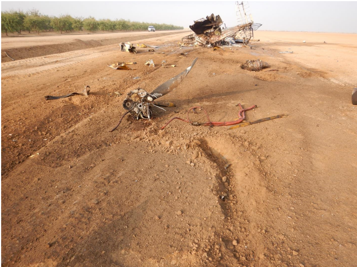
Figure 3-Debris field, propeller ground scars and engine sections.
