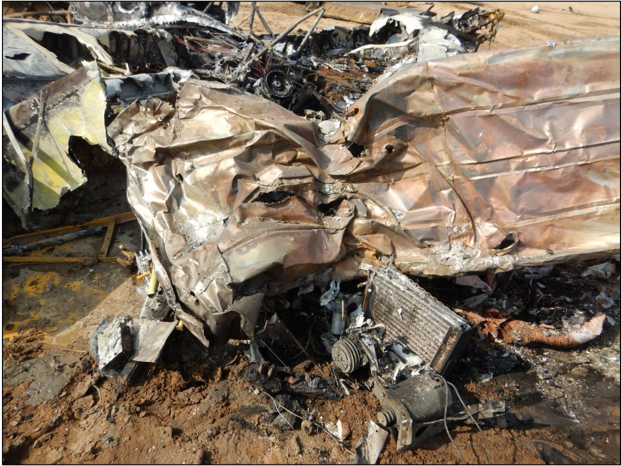
Figure 6-Lower side of fuselage, impact damage.
