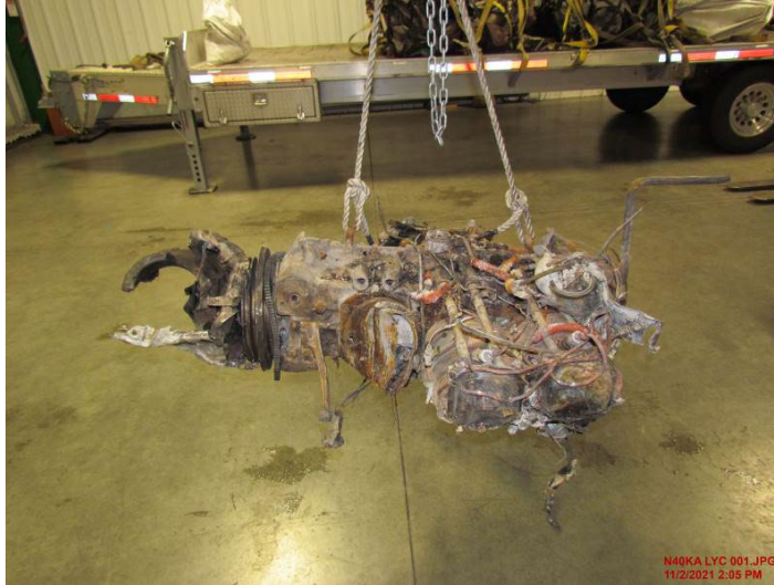
Figure 3: Post-accident view of the engine
