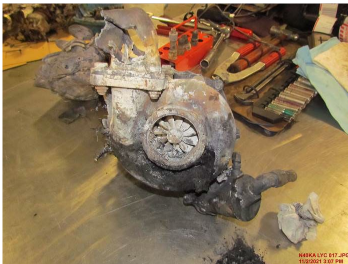
Figure 4: Post-accident view of the turbo charger
