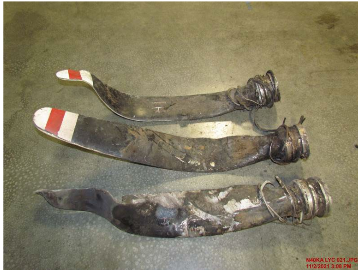
Figure 2: Post-accident view of the propeller blades
