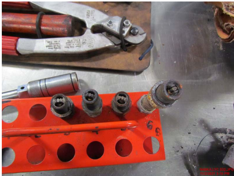
Figure 5: View of the intact spark plugs
